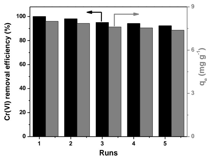
**Figure 6.** The reusability of the NMC for the Cr(VI) removal in this work, condition: [Cr (VI)] = 20 mg L<sup>-1</sup>, pH = 7.0, adsorbent dosage: 50.0 mg, volume: 20 mL, treatment time: 10 min.
