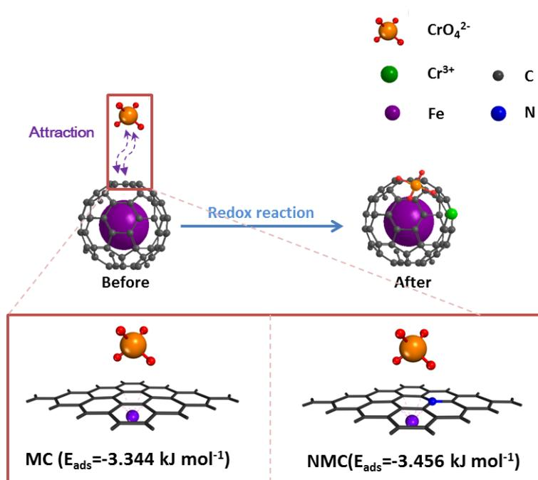
**Figure 10.** Proposed adsorption mechanism of magnetic carbons for the Cr(VI) removal.
