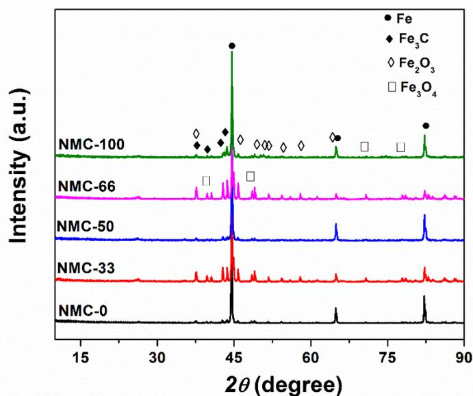
**Figure 2.** XRD patterns of magnetic adsorbents used in this study.
