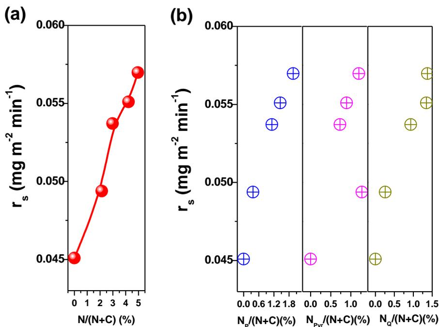
**Figure 9.** Dependences of Cr(VI) removal rate on the amounts of nitrogen: (a) gross N content; (b) N functionalities,  $N_p$ : pyridinic group;  $N_{pyr}$ : pyrrolic group;  $N_q$ : graphitic N group.
