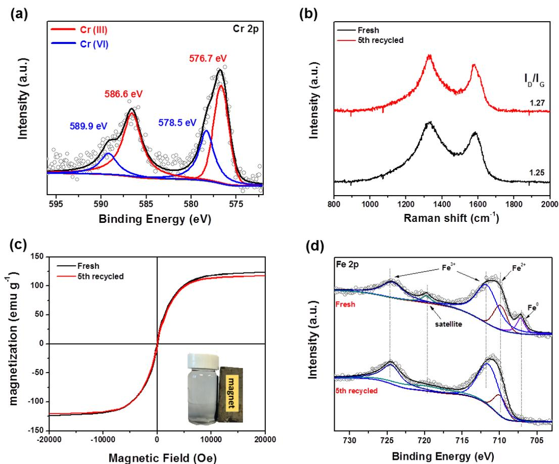
**Figure 7.** (a) Raman spectral, (b) magnetization and (c) Fe 2p XPS spectra of the fresh and 5th recycled samples, (d) Cr 2p XPS result of the 5th recycled samples.
