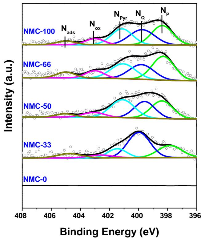
**Figure 3.**  $N_{1s}$  XPS spectra of the magnetic adsorbents used in this work.
