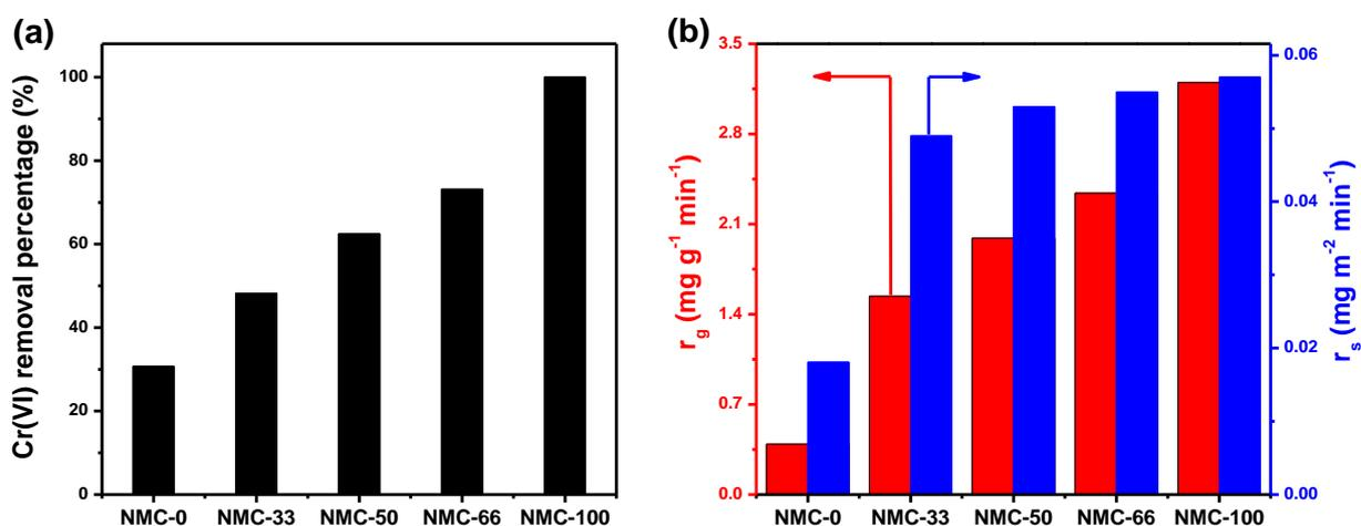
**Figure 8.** [a] Performance of different adsorbents on the Cr(VI) removal, condition:  $[\text{Cr}(\text{VI})] = 20 \text{ mg L}^{-1}$ ,  $\text{pH} = 7.0$ , adsorbent dosage:  $50.0 \text{ mg}$ , volume:  $20 \text{ mL}$ , treatment time:  $10 \text{ min}$ ; [b] Removal rate of Cr(VI) per gram and per  $\text{m}^2$  of catalyst surface of adsorbent based on the treatment within  $2.5 \text{ min}$ .
