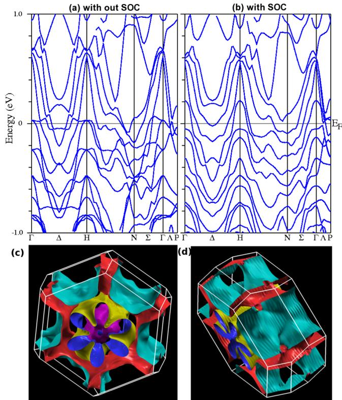
FIG. 5. (Color online) Electronic band structure of  $\text{LaIr}_3$ . (a) Band-structure with-out SOC and (b) band-structure with SOC. Complex Fermi surface shows on (c) and (d) for merged bands.
