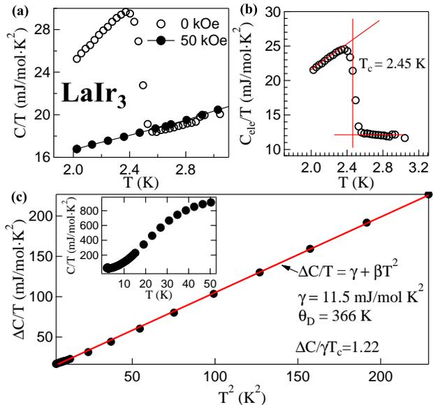
FIG. 3. (Color online) Analysis of heat capacity of  $\text{LaIr}_3$ . (a) Heat capacity at zero (open symbol) and 5 T (Tesla) (closed symbol) applied field. (b) The electronic heat capacity jump, which can be used to extract  $T_c$  by using the equal-area construction method. (c) The 5 T heat capacity data. The solid line shows the fit with equation  $\frac{C}{T} = \gamma + \beta T^2$ . The upper left inset shows the zero-field heat capacity as a function of temperature.
