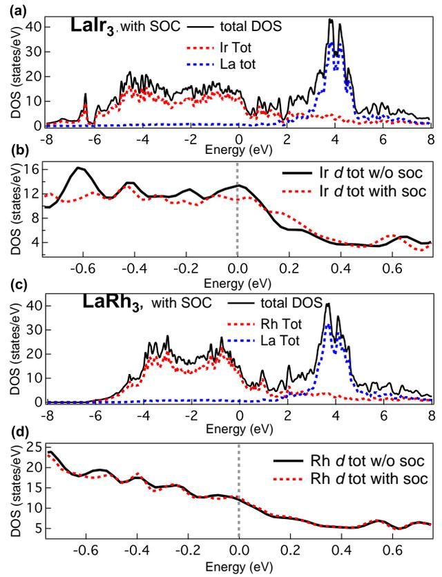
FIG. 4. (Color online) The density of states of  $LaIr_3$  and  $LaRh_3$ . (a) The total DOS of  $LaIr_3$ , as well as the contributions of La and Ir states respectively. Spin-orbit coupling (SOC) is included. (b) Ir  $d$ -band DOS with and without SOC. (c) The total DOS of  $LaRh_3$ , as well as the contributions of La and Rh states respectively. Spin-orbit coupling (SOC) is included. (d) Rh  $d$ -band DOS with and without SOC.
