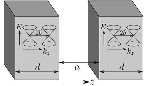
FIG. 1. The setup we will consider here is two Weyl semimetals separated by a distance  $a$  in vacuum, and with distance between Weyl cones  $2\mathbf{b}$  in  $k$ -space (split in the  $z$ -direction).
