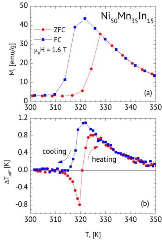
Figure 3: Temperature dependence of magnetization and  $\Delta T_{ad}$  in 1.6 T field in the vicinity of martensitic transition for  $Ni_{50}Mn_{35}In_{15}$  sample.
