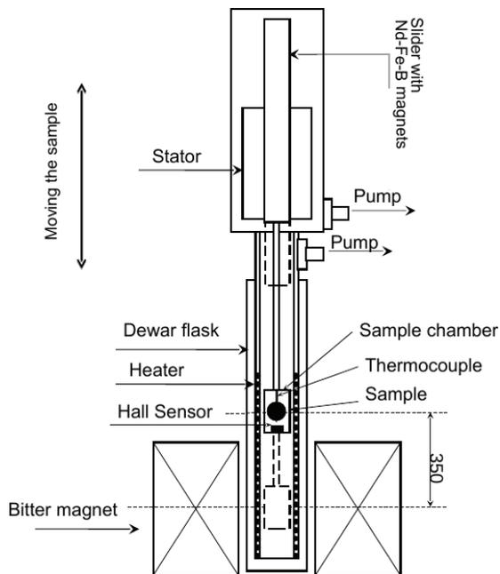
Figure 1: Schematic overview of high field setup for  $\Delta T_{ad}$  measurements developed by Yu. S. Koshkid'ko and J. Cwik.
