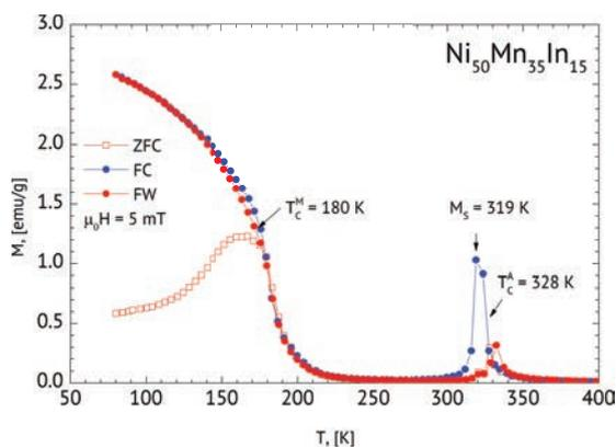
Figure 2: Temperature dependence of magnetization in 5 mT field for  $\text{Ni}_{50}\text{Mn}_{35}\text{In}_{15}$  sample.
