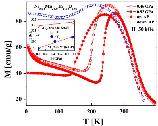
Fig. 5 ZFC and FCC  $M(H)$  curves of  $\text{Ni}_{50.51}\text{Mn}_{34.34}\text{In}_{14.14}\text{B}_{1.01}$  obtained at  $H=50$  kOe and at different applied hydrostatic pressures. Inset: Variation of the transition temperatures  $T_C$  and  $T_M$ , open and closed symbol, respectively, with applied pressure.
