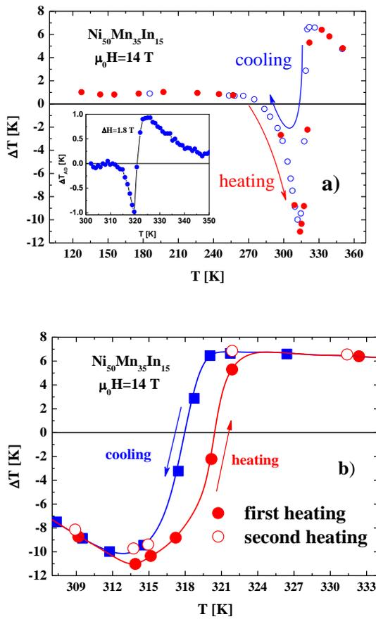
**Fig.4** (a) Temperature dependence of the adiabatic temperature change  $\Delta T_{ad}$  in  $\text{Ni}_{50}\text{Mn}_{35}\text{In}_{15}$  alloys in an applied magnetic field of 14 T (inset shows the same for  $H = 1.8$  T, the data were taken from Ref. [12]) in the vicinity of the martensitic transformation; (b) The corresponding curves for a narrow temperature range in the area of temperature hysteresis.
