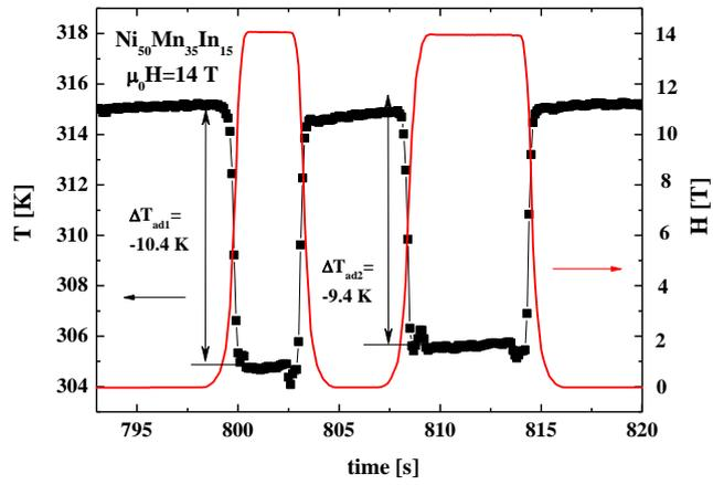
**Fig.5** The adiabatic temperature (left panel) and external magnetic field (right panel) changes as a function of time obtained for a maximum value of  $\Delta H=14$  T at the first and subsequent magnetization cycles at  $T = 315$  K.
