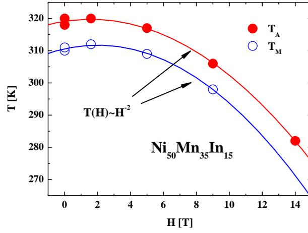
**Fig. 3** The field dependence of the martensitic transition temperatures.
