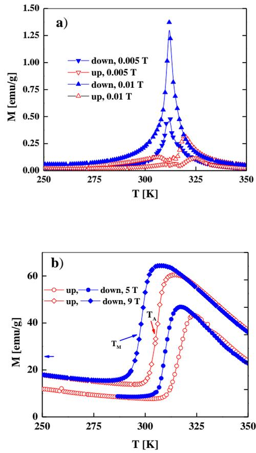
**Fig. 2** ZFC and FCC  $M(T)$  curves for (a) low applied magnetic fields and (b) strong magnetic fields.  $T_M$  and  $T_A$  are the temperatures of the direct and inverse martensitic transformations.
