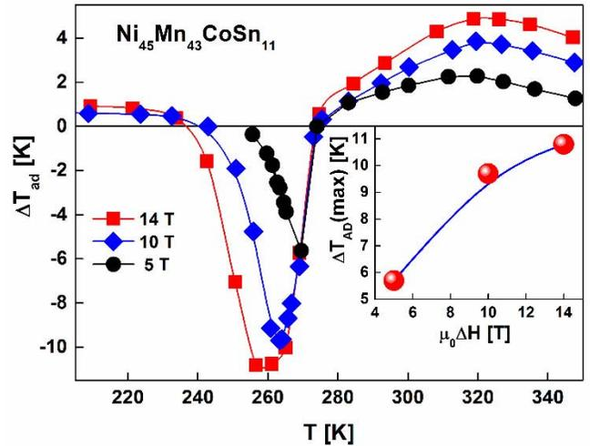
Fig. 2. Adiabatic temperature change ( $\Delta T_{\text{ad}}$ ) of  $\text{Ni}_{45}\text{Mn}_{43}\text{CoSn}_{11}$  as a function of temperature for different  $\mu_0\Delta H$  values obtained during the first heating. Inset: maximum  $\Delta T_{\text{ad}}$  at MST at different magnetic fields.
