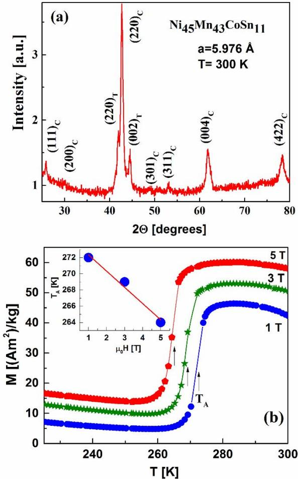
Fig. 1. (a) Room-temperature XRD of  $\text{Ni}_{45}\text{Mn}_{43}\text{CoSn}_{11}$  Heusler alloy. The indices “T” and “C” are used to indicate the martensitic tetragonal and austenitic cubic phases, respectively. (b)  $M(T)$  curves obtained at magnetic fields up to 5 T. The phase transition temperatures ( $T_A$ ) from low magnetization martensitic to ferromagnetic austenitic phases are indicated by the arrows.
