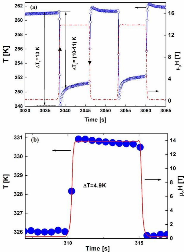
Fig. 4. (a) Adiabatic temperature change of  $\text{Ni}_{45}\text{Mn}_{43}\text{CoSn}_{11}$  for the first and second applications of magnetic field in the temperature region near the MST.  $\Delta T_1$  is the initial value of the adiabatic temperature change, and  $\Delta T_2$  is the value of the adiabatic temperature change after relaxation. (b)  $\Delta T_{\text{ad}}$  of  $\text{Ni}_{45}\text{Mn}_{43}\text{CoSn}_{11}$  near the Curie temperature.
