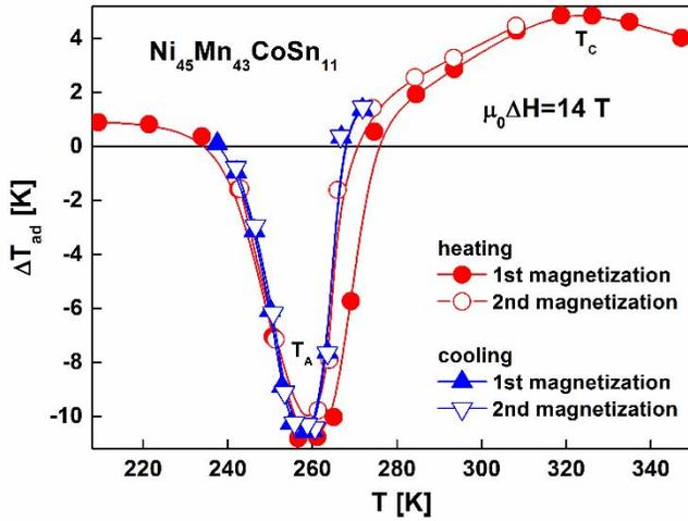
Fig. 3. Adiabatic temperature change of  $\text{Ni}_{45}\text{Mn}_{43}\text{CoSn}_{11}$  as a function of temperature ( $T$ ) for  $\mu_0 \Delta H = 14$  T during two heating and cooling cycles.
