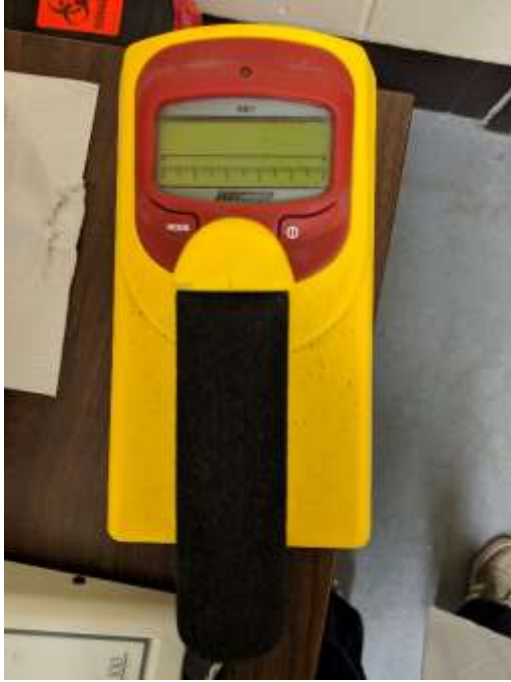
Figure 2.4. Fluke 451B ion chamber survey meter used to perform exposure rate measurements in units of mR/hr.
