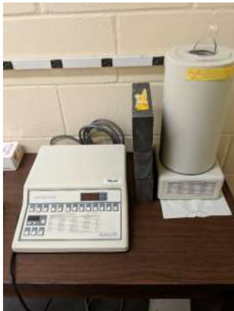
Figure 2.7. Biodex Atomlab 100 dose calibrator used to measure excreted activity.
