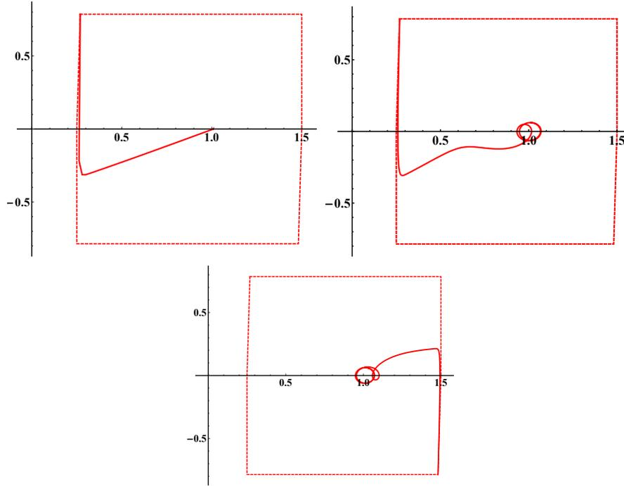
Figure 2.6. States  $(\rho(t), \phi(t)) = (\tilde{q}_1(t) + \rho_0, \tilde{q}_2(t))$  Staying in Robustly Forwardly Invariant Set on Time Interval  $[0, 20]$  Without Disturbances (Upper Left) and  $\delta(t) = 2.5 \sin(t)$  (Upper Right and Bottom).
