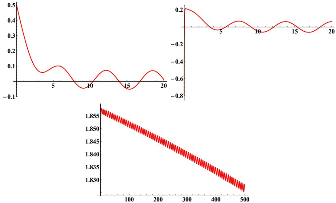
Figure 2.5. Plots from Augmented Error Dynamics (2.66) with Initial Value  $(\tilde{q}(0), \tilde{\kappa}_0(0)) = (0.5, -\pi/4, 0.15)$  and  $\delta(t) = 2.5 \sin(t)$ . (Top Left)  $\tilde{q}_1(t) = \rho(t) - \rho_0$ , (Top Right)  $\tilde{q}_2(t) = \phi(t)$ , and (Bottom)  $\hat{\kappa}(t)$ .
