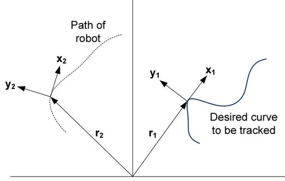
Figure 2.1. Positions and frames for the vehicle  $(\mathbf{r}_2, \mathbf{x}_2, \mathbf{y}_2)$  and shadow point  $(\mathbf{r}_1, \mathbf{x}_1, \mathbf{y}_1)$  of our vehicle/shadow point pair. Let  $\mathbf{r} = \mathbf{r}_2 - \mathbf{r}_1$  be the vector pointing from the shadow point on the curve to the current position of the vehicle. We assume that
