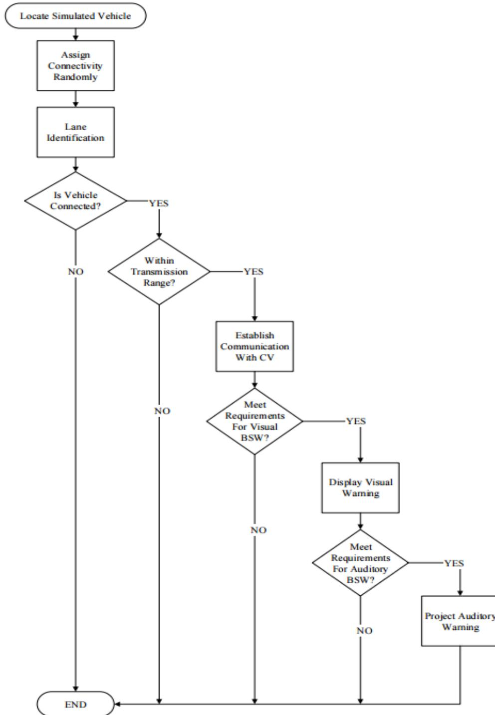
FIGURE 3 Blind spot warning (BSW) calling process.
