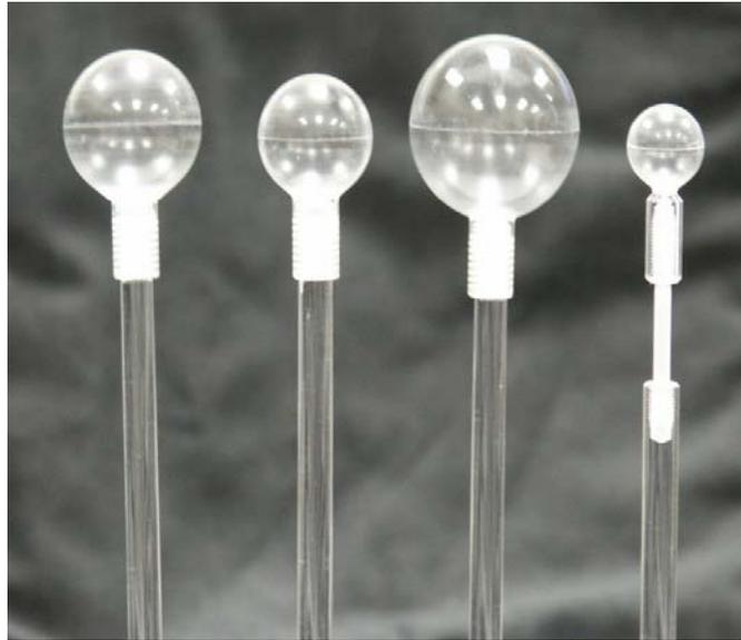
Figure 7: Hot Sphere phantom comprising hollow sphere set.
