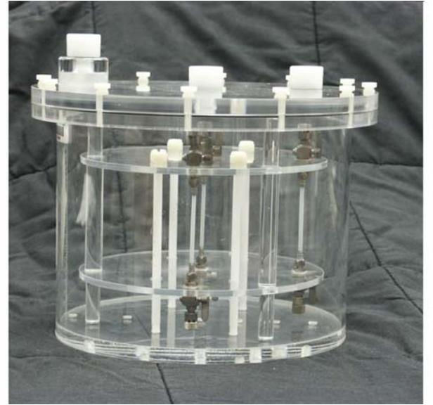
Figure 6: (a) Triple-line phantom and (b) Triple-line phantom mounted inside the ECT cylinder.
