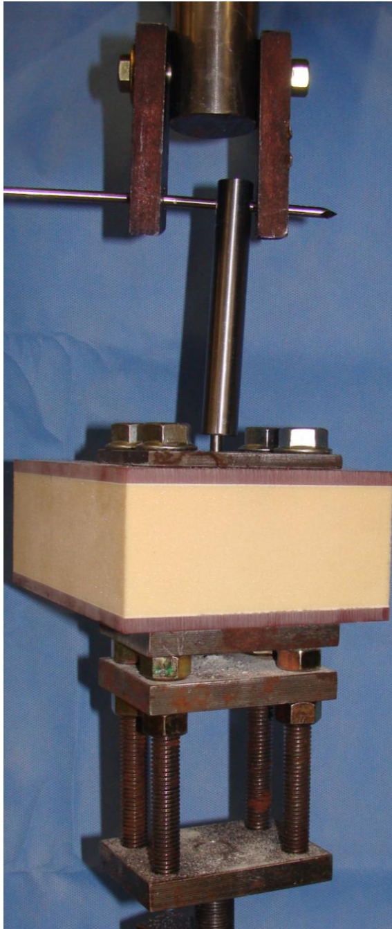
Figure 3.3. Photograph showing the AP pullout test construct in the MTS.
