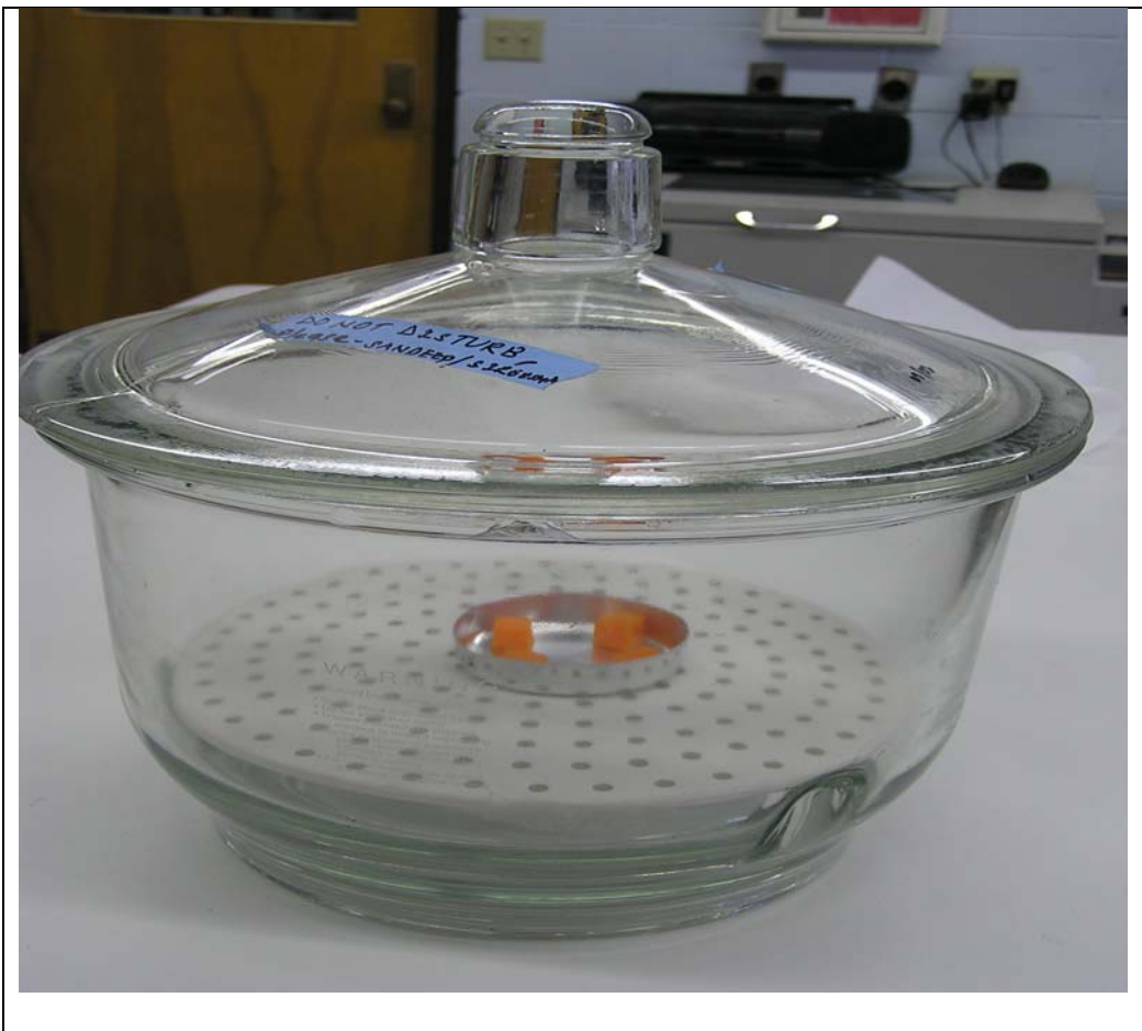
Figure # 2. Dessicator with the samples
