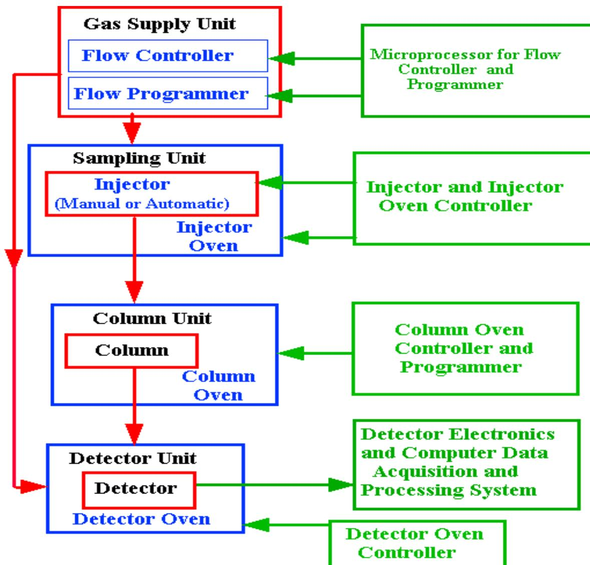
Figure 1. Gas Chromatograph Functional Diagram (Scott)
