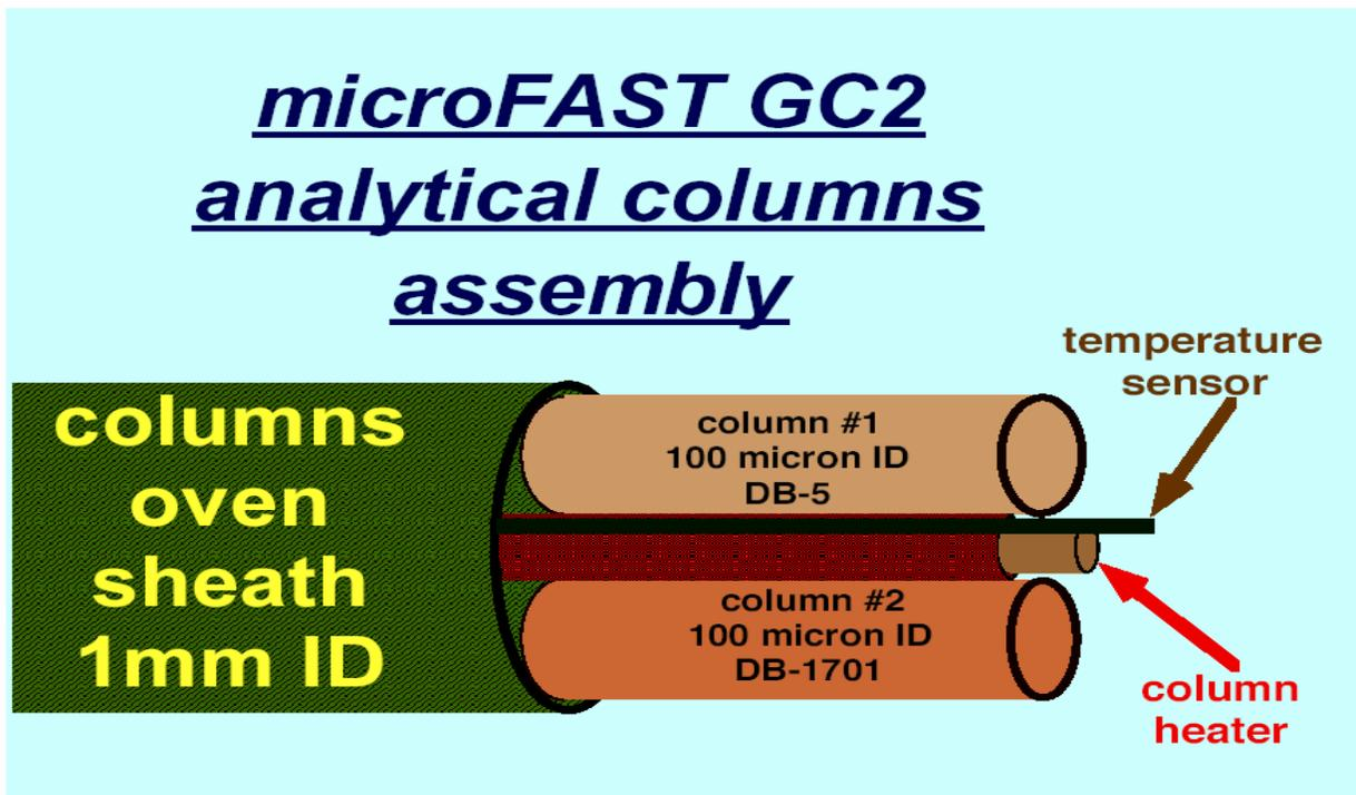
Figure 2: Heating element incorporation into column assembly. (ASI)
