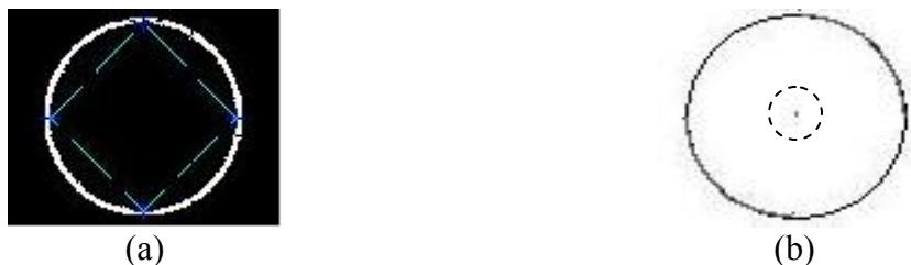
Figure 5.7. Comparison of results between: (a) our new initialization algorithm and (b) the center-of-divergence method (solid line: circle object, dashed line: initial contour).
