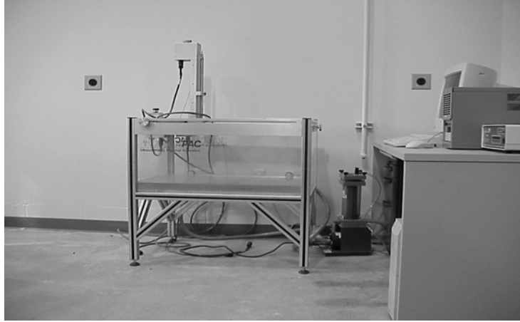
Figure 5.6. Ultrasonic imaging equipment for nondestructive evaluation of materials.
