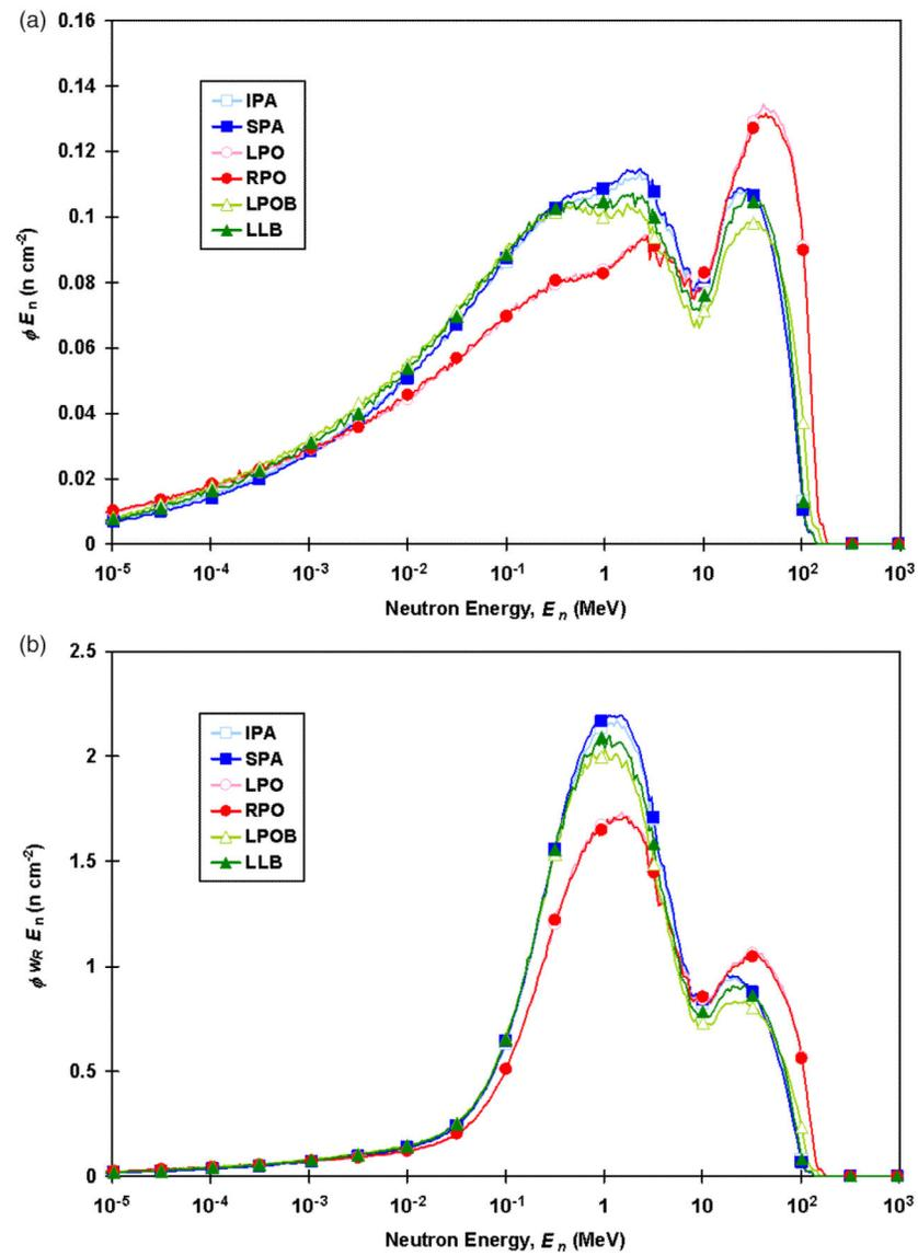
**Figure 2.** External neutron spectral fluence (a) and external neutron spectral fluence weighted by the analytical expression of the radiation weighting factor (b) for each field. Abbreviations used are the same as those in table 1.
