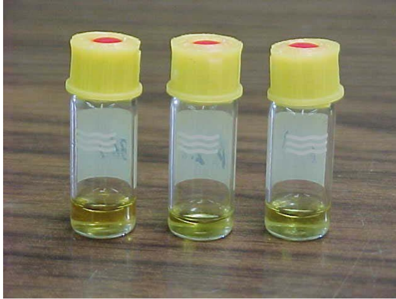
Fig. 2.5 FAME samples ready for GC analysis
