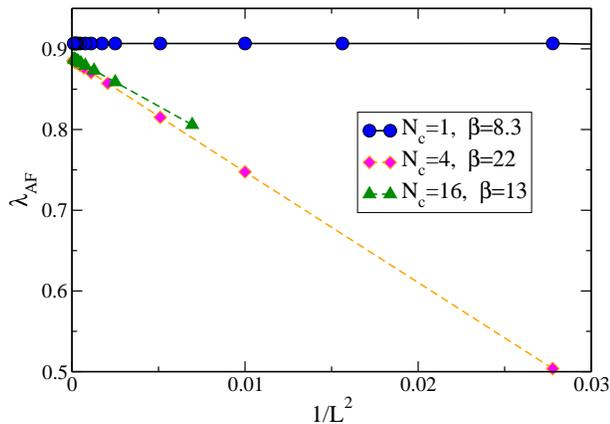
FIG. 8: (Color online) The  $L$  dependence of the leading eigenvalue for different DCA clusters. The parameters used are  $U = 8t$ ,  $\langle n \rangle = 1$ ,  $\Sigma_{dual} = 0$  and  $\beta = 4t/T$ . The nice linear dependence of  $1/L^2$  can be readily observed, which is due to the periodic boundary conditions used in the dual-fermion calculation.
