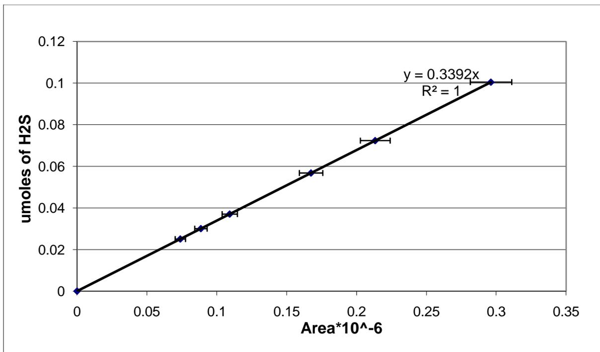
**Figure A. 2 Calibration for H<sub>2</sub>S**
