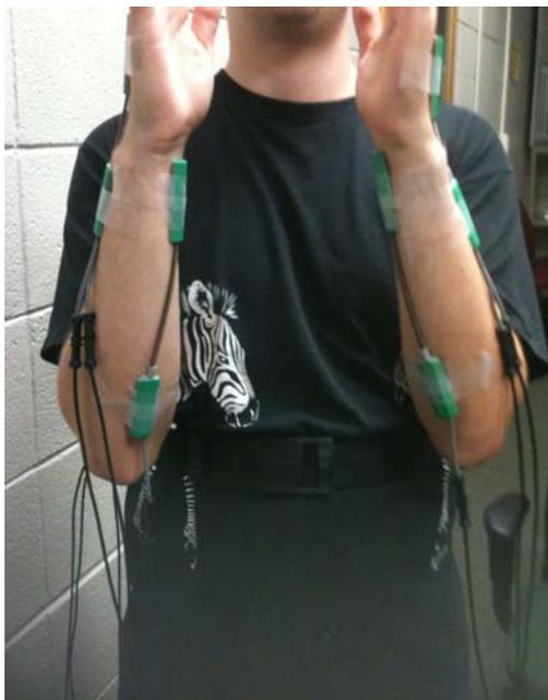
Figure 3.2: Front view of placement of both electrogoniometers and torsiometers on both lower arms
