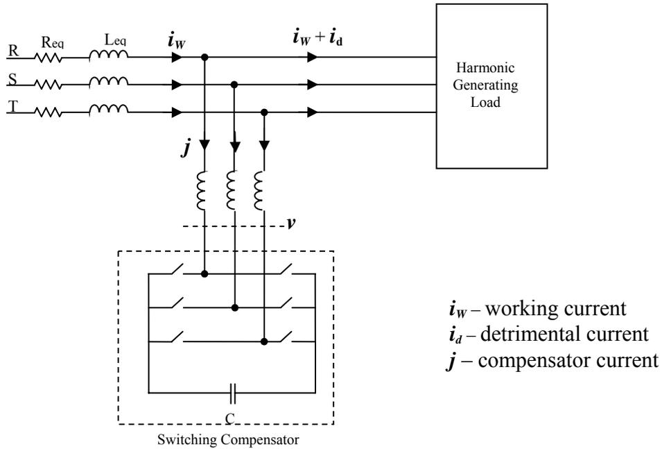
Figure 4.1 Compensator Showing Working and Detrimental Current
