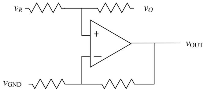
Figure 7.3 OP-AMP Circuit Used to Insert DC Offset
