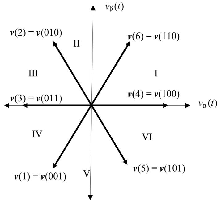
Figure 5.3 State Vectors On the  $\alpha\beta$  Plane
