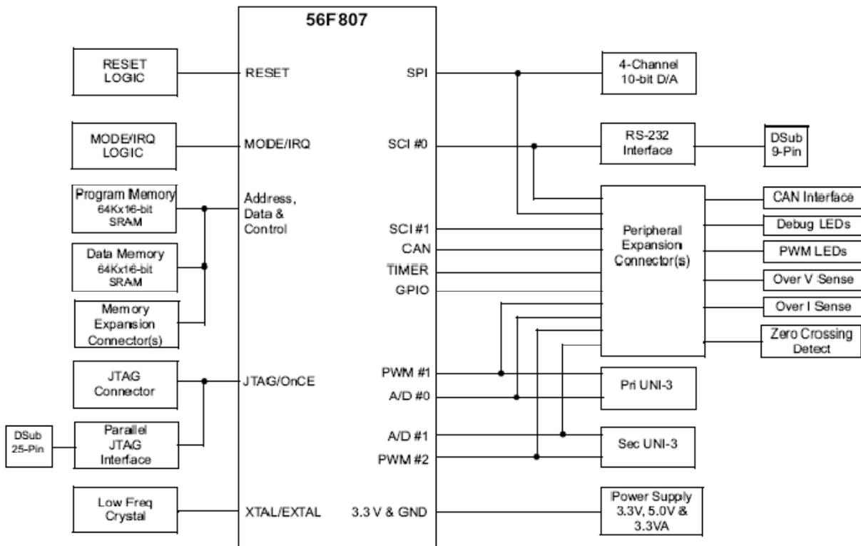
Figure 7.1 Basic Structure of the 56F807 DSP Board [20]
