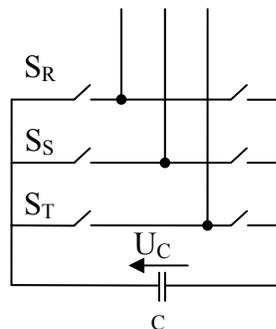
Figure 5.8 Names of the Power Switches
