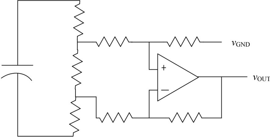
Figure 7.4 OP-AMP Circuit to Calculate Capacitor Voltage
