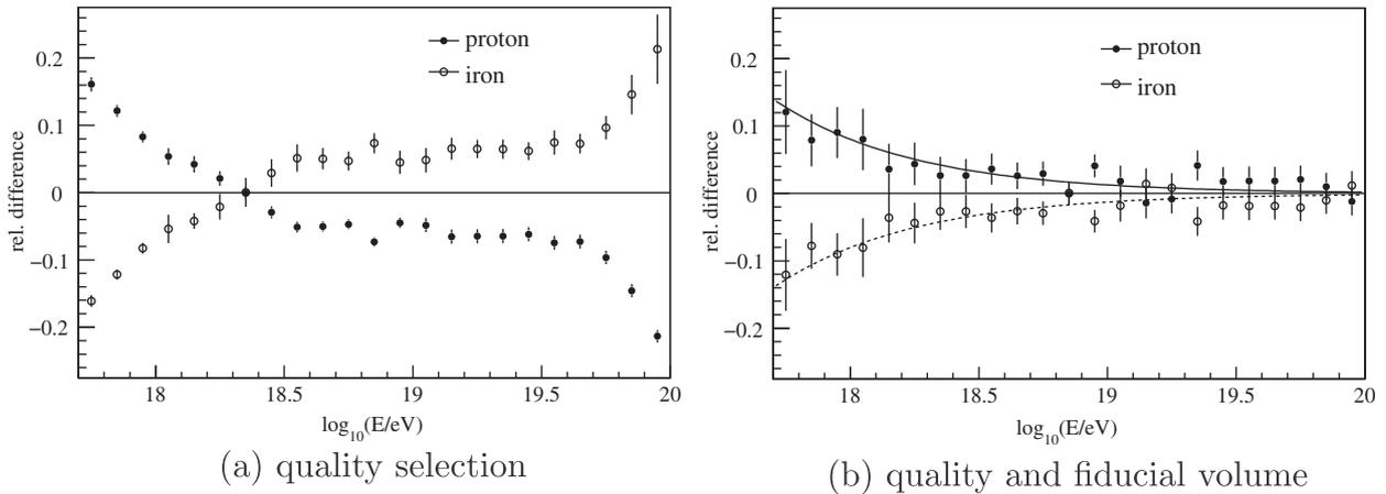
**Fig. 6.** Relative difference between proton and iron exposure with respect to a mean composition exposure, as obtained from the Time Dependent Detector Simulation. In the left panel the dependence on the primary mass is clearly visible. In the right panel this difference is strongly reduced by the fiducial volume cut.
