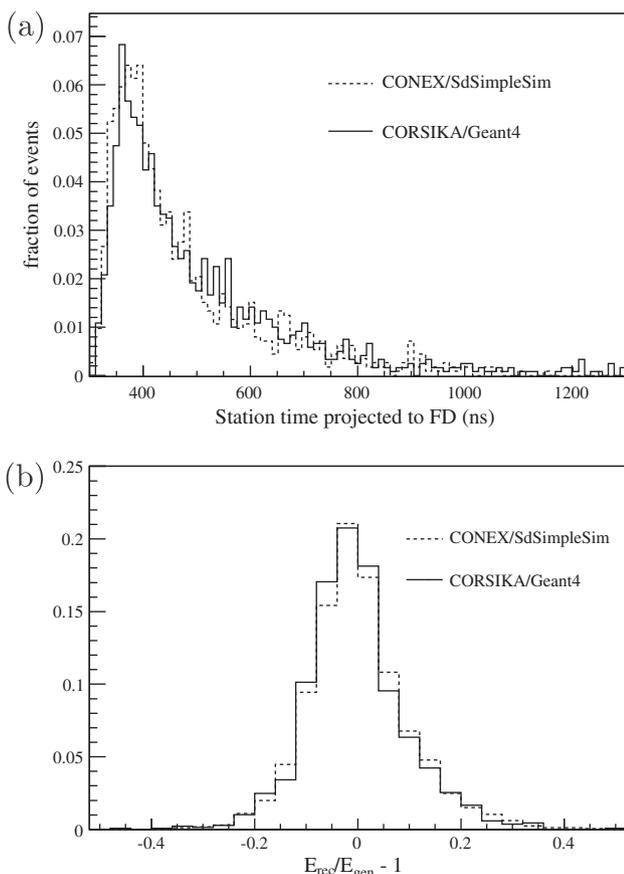
**Fig. 5.** Comparison between CORSIKA/Geant4 simulations and the fast CONEX/SdSimpleSim approach. (a) Distribution of the time at which the SD station is triggered. (b) Difference between the simulated and the reconstructed energies using the hybrid technique. The figures refer to events at  $\log_{10}(E/\text{eV}) = 18.5$ .
