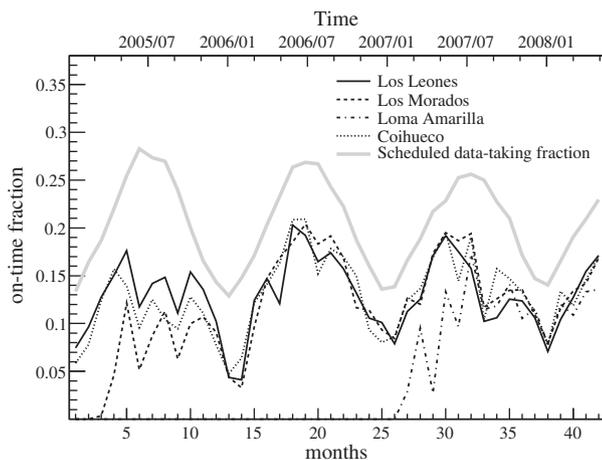
**Fig. 3.** Time evolution of the average hybrid on-time fraction during the construction phase of the Pierre Auger Observatory. Both the seasonal modulation and the starting of commissioning phases of the different FD-sites are visible. Gray line represents the scheduled data-taking time fraction limited to the nights with moon-fraction lower than 60%.
