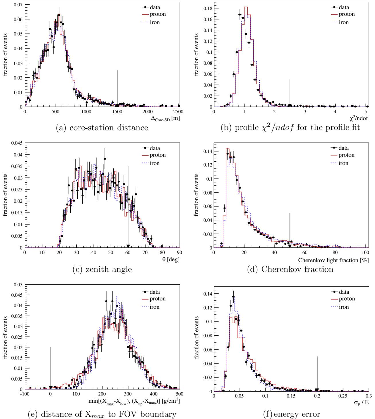
**Fig. 8.** Examples showing the agreement between simulation and data. Proton and iron primaries are shown separately for the simulated data. For each figure all quality and fiducial cuts are applied except the one related to the variable shown. The arrow denotes the selection cut on this variable.
