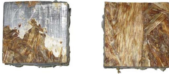
**Figure 4. IB glue bond failure. Block at left has shows approximately 60 percent adhesive failure. Block at right shows proper adhesion and sample failure.**
