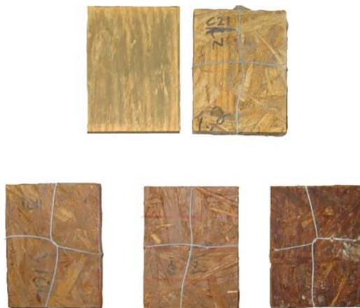
**Figure 15. Samples after mold testing. Top row: untreated solid pine, untreated pine strandboard. Bottom row: 10 percent PD-112, 17 Percent PD-112 and 23 Percent PD-112.**
