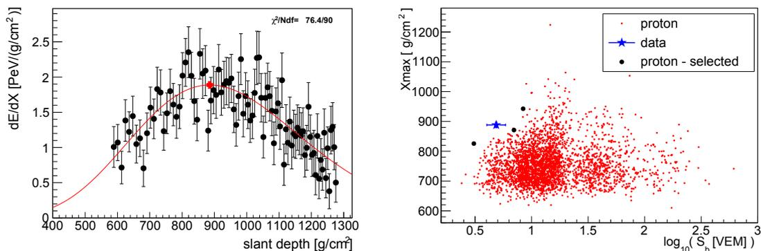
**Figure 4.** Left: longitudinal profile and Gaisser-Hillas fit of one of the selected photon candidates (ID 6691838). Right: correlation plot of  $X_{\max}$  and  $S_b$  for the candidate (blue star) and dedicated proton events simulated with the same energy, geometry and detector configuration as the real event (red dots). Three out of 3000 simulated proton showers are selected as photon candidates (black circles).
