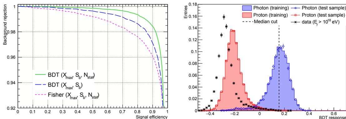
**Figure 3.** Left: curve of the background rejection efficiency against the signal efficiency for different algorithms and observables. Right: distribution of the Boosted Decision Tree observables for signal (photon, blue), background (proton, red) and data (black). For simulations both the training and the test samples are shown. The cut at the median of the photon distribution is indicated by the dashed line. QGSJET-II-04 used as high-energy hadronic interaction model.
