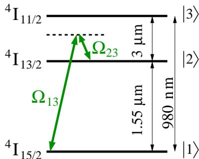
FIG. 3: Schematic level diagram of  $\text{Er}^{3+}$  ion discussed in the context of the deterministic STIRAP pumping scheme. Using the technique of STIRAP, the population transfer to the level  $|2\rangle$  does not depend on the branching ratio and can be made with unit efficiency.
