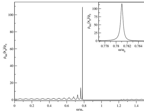
FIG. 4: Normalized local mode density at the ion position for a 29-layer stack with  $n_1 = 1$ ,  $n_2 = 2$ . The ion is placed in the middle of the dielectric slab situated halfway between the longitudinal boundaries of the structure. The inset shows an expanded view of the spectral region surrounding the band edge frequency. The line-width of the  $\text{Er}^{3+}$  ion itself is about 0.0001 in these dimensionless units [26].
