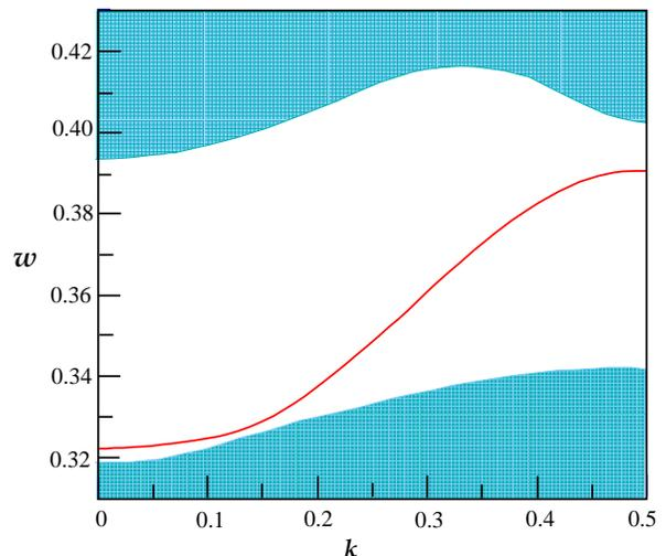
FIG. 2: Schematic dispersion relation of a PBG heterostructure similar to one presented in Fig. 1 for propagation along the waveguide direction ( $w = \omega a/2\pi c$ ,  $k = k_{\parallel} a/2\pi$ ). By removing one row of rods, the linear defect supports a single waveguided mode and, by appropriately choosing unit cell size, the mode will experience a sharp cutoff in the spectral region around the  $|2\rangle \rightarrow |1\rangle$  transition frequency.
