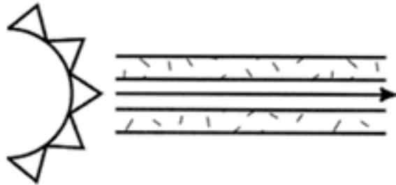
Figure 2-1: Single Mode Fiber: Single path through fiber.
