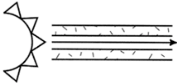
Figure 2-1: Single Mode Fiber: Single path through fiber.
