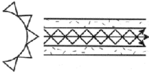
Figure 2-2: Multimode fiber: Multiple paths through the fiber.
