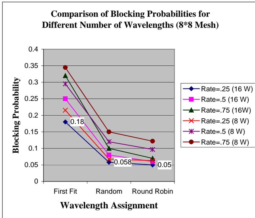
Figure 4-4: Blocking Probability for Different Number of Wavelengths.
