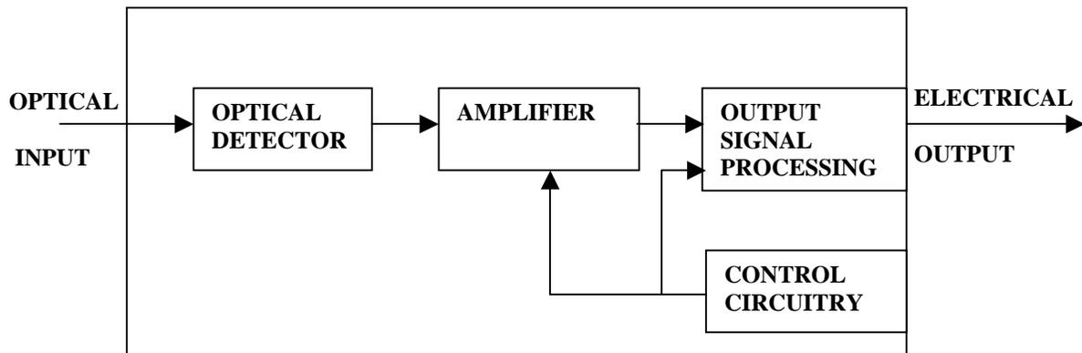
Figure 2-4: Block diagram of a fiber optic receiver.
