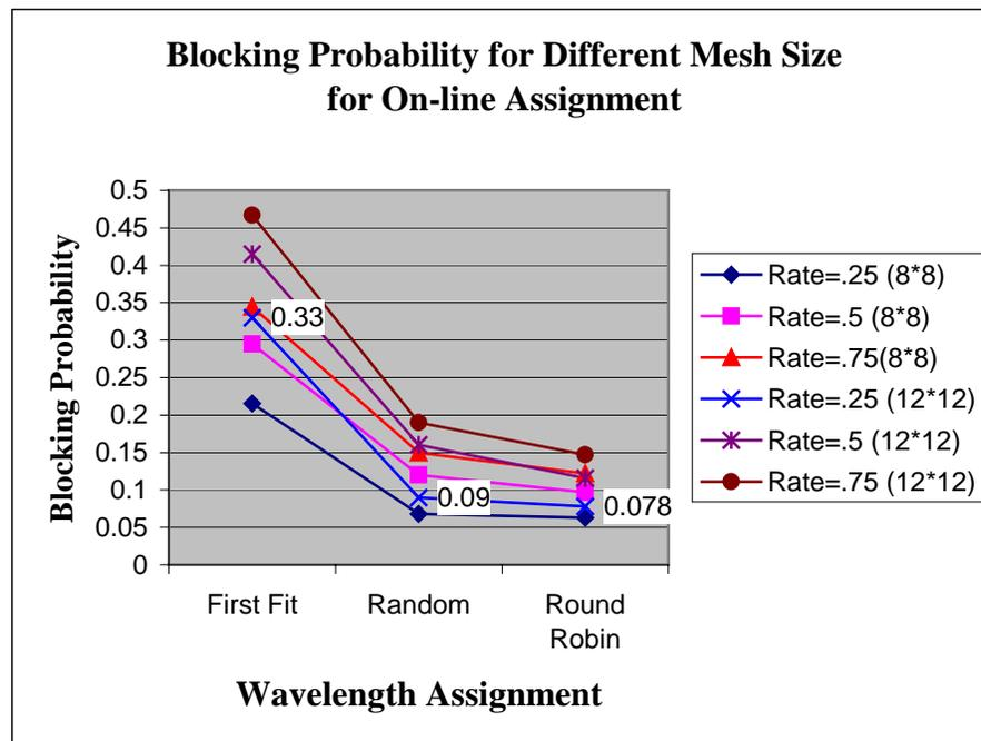
Figure 4-5: Blocking Probability for Different Mesh Dimensions.
