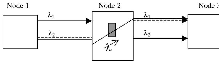
Figure 2-5: Figure showing the use of wavelength converter.
