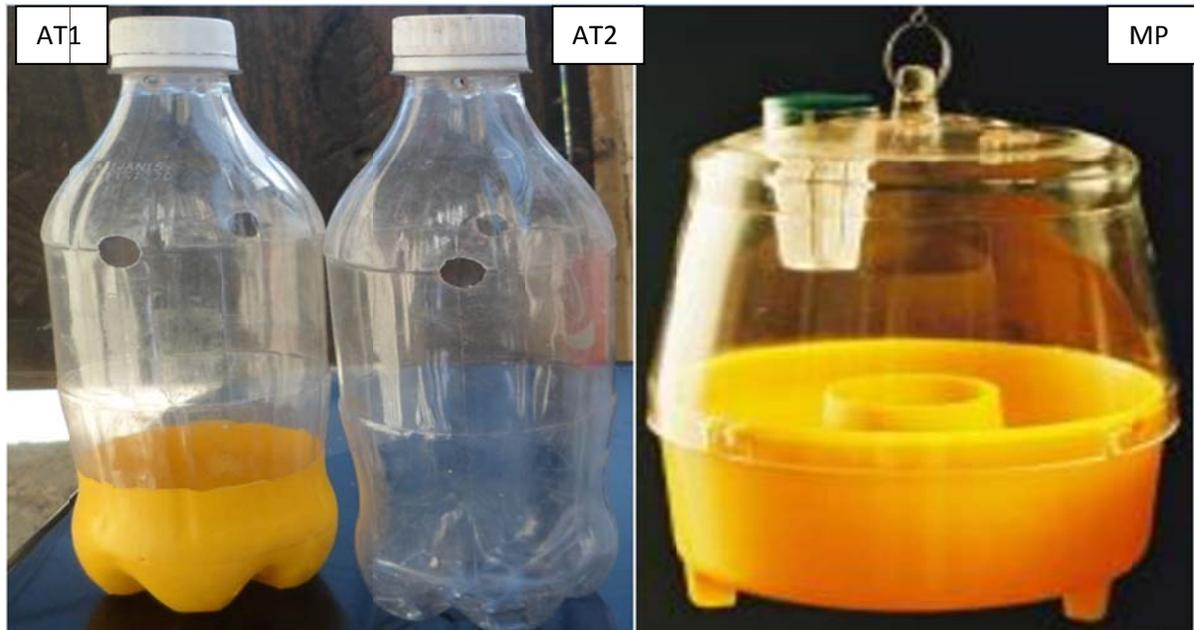
Fig. 2.1: Trap models developed and used for the study: AT1, yellow bottom artisanal trap; AT2, clear artisanal trap; and MP, Commercial McPhail trap.
