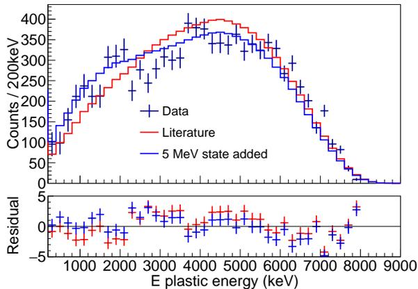
FIG. 8: (Color Online) The  $\beta$ -energy spectrum for  $\beta$ -ion coincidences compared to simulations which include the decay scheme from the Nuclear Data Sheets [16] with  $a_{\beta\nu} = 1$  (red) combined with a single fictitious allowed Gamow-Teller transition with  $a_{\beta\nu} = -1/3$  to a 5-MeV (blue) excited state which decays directly to the ground state by a single  $\gamma$  ray, scaled to match counts above 200 keV.
