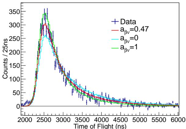
FIG. 6: (Color Online) The measured  $^{134}\text{Sb}$  TOF spectrum compared to simulations using the decay scheme in Ref. [16] with different  $a_{\beta\nu}$  values. The value which matches  $R_{180/90}=9.33$  from the data is  $a_{\beta\nu}=0.47$  and the resulting TOF distribution is shown in red. The TOF spectra for  $a_{\beta\nu}=0$  (cyan) and  $a_{\beta\nu}=1$  (green) are also shown and result in  $R_{180/90}$  values that are inconsistent with the data.
