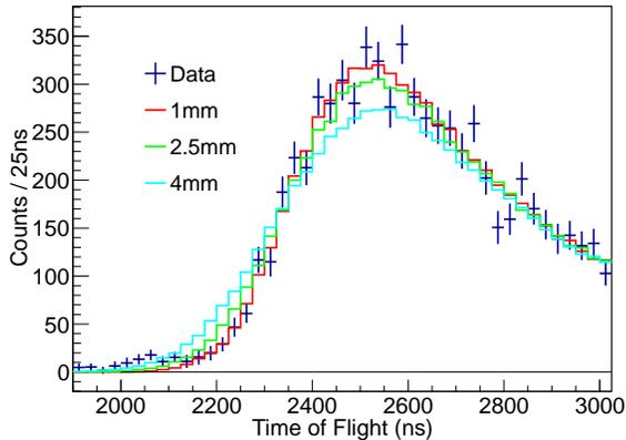
FIG. 5: (Color Online) The rising edge of the  $^{134}\text{Sb}$  decay TOF compared with three simulated cloud sizes, labeled by the FWHM of the Gaussian distribution used. The 1 mm (red) simulation is scaled to match counts between 2400–2600 ns, and the 2.5 mm (green) and 4 mm (cyan) are shown with the same number of  $\beta$ -ion coincidences as the 1 mm simulation.
