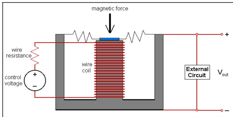
Figure 2.3. A diagram of an electromagnetic micro-relay
