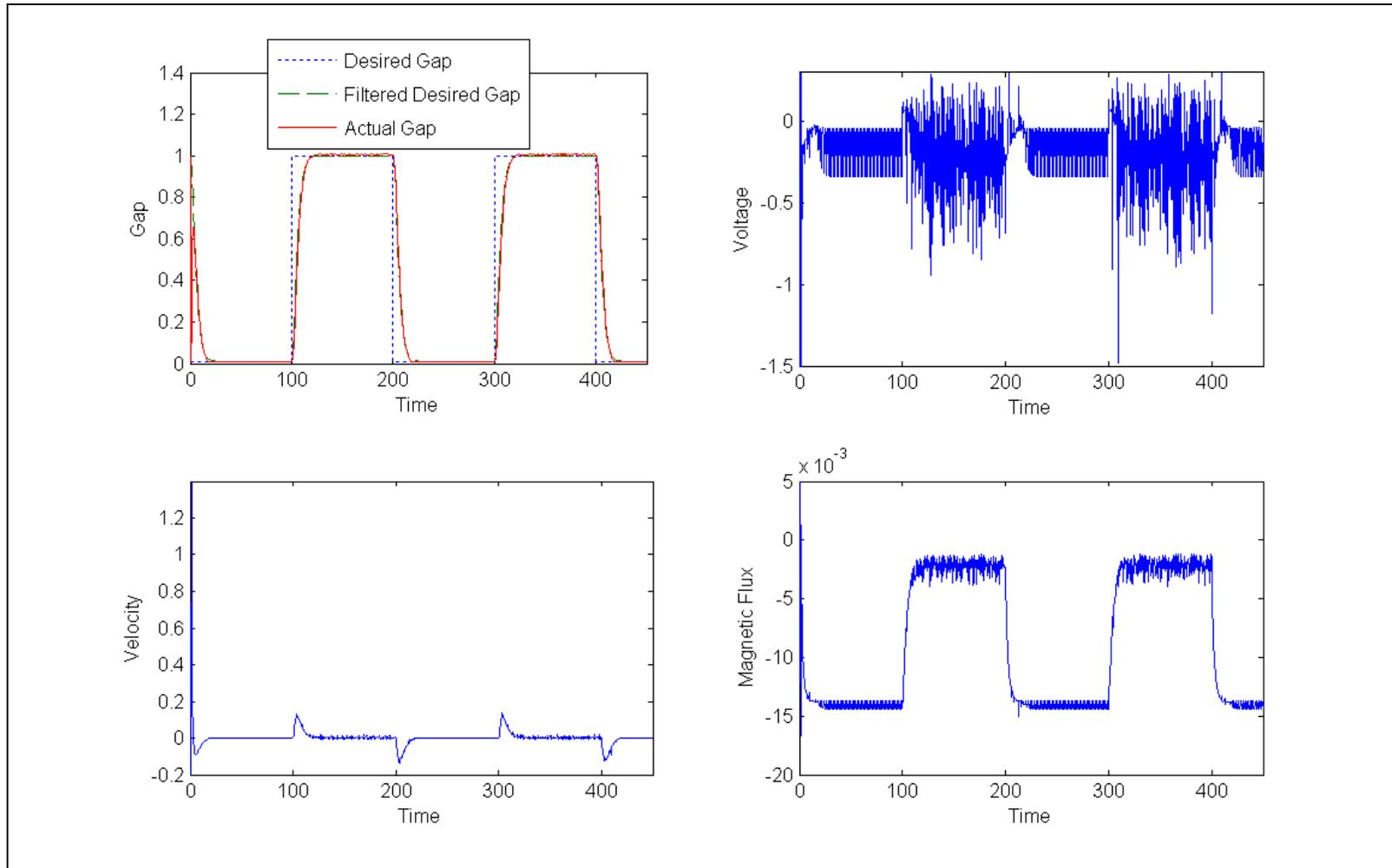
Figure 5.2. Electromagnetic micro-relay operation with feedback linearization-based control
