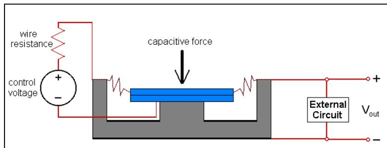
Figure 2.1. A diagram of an electrostatic micro-relay
