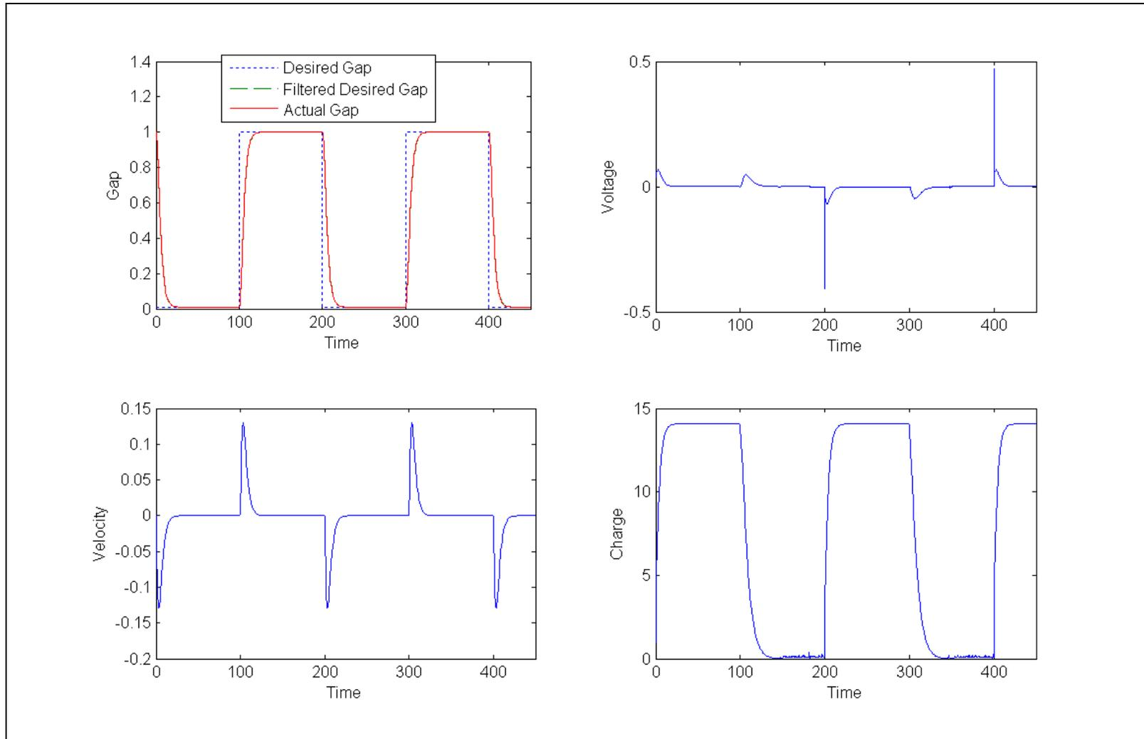
Figure 5.1. Electrostatic micro-relay operation with feedback linearization-based control
