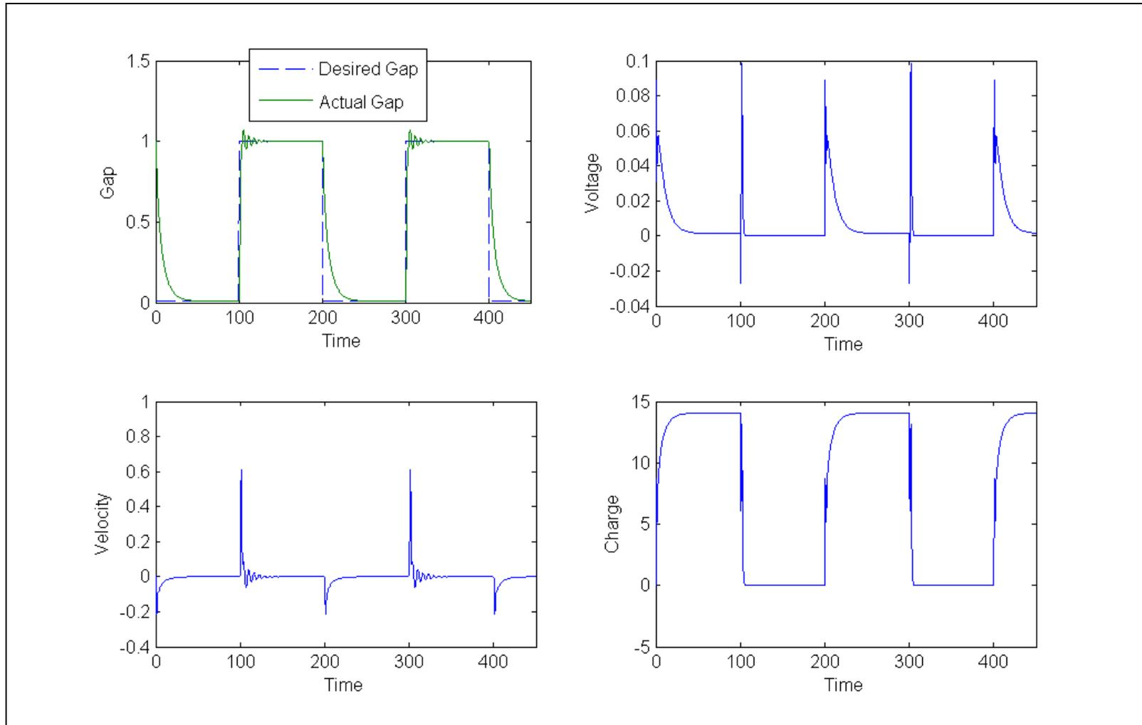
Figure 4.1. Electrostatic micro-relay operation with Lyapunov-based control
