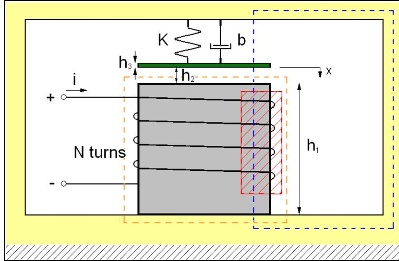
Figure 2.4. A simple electromagnetic micro-relay model
