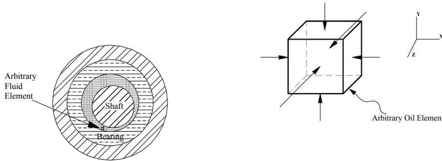
**Figure 3.2 identifies the fluid element and the pressure acting on the element within the journal bearing**
