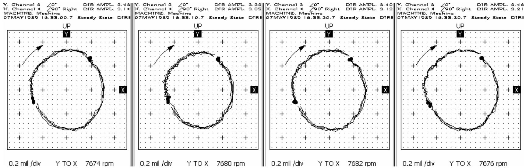
Figure 6.15: Orbits of rotor #3 prior to the damage.
