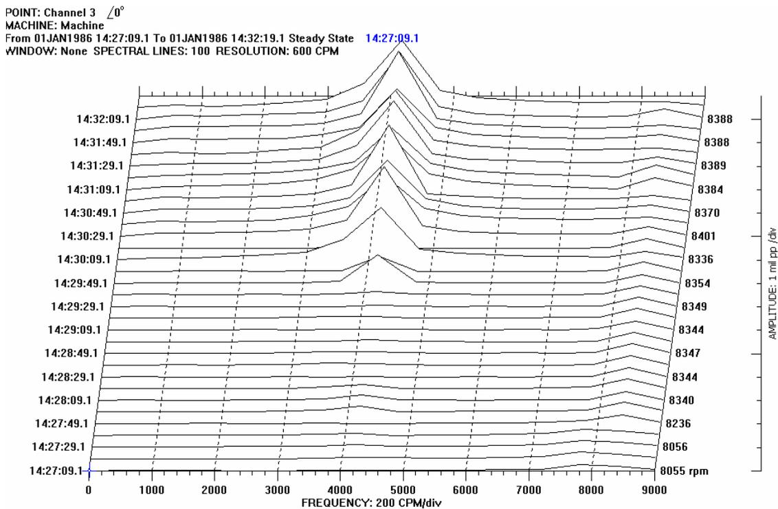
**Figure 6.10: The waterfall plot of the experimental threshold of rotor #4**
