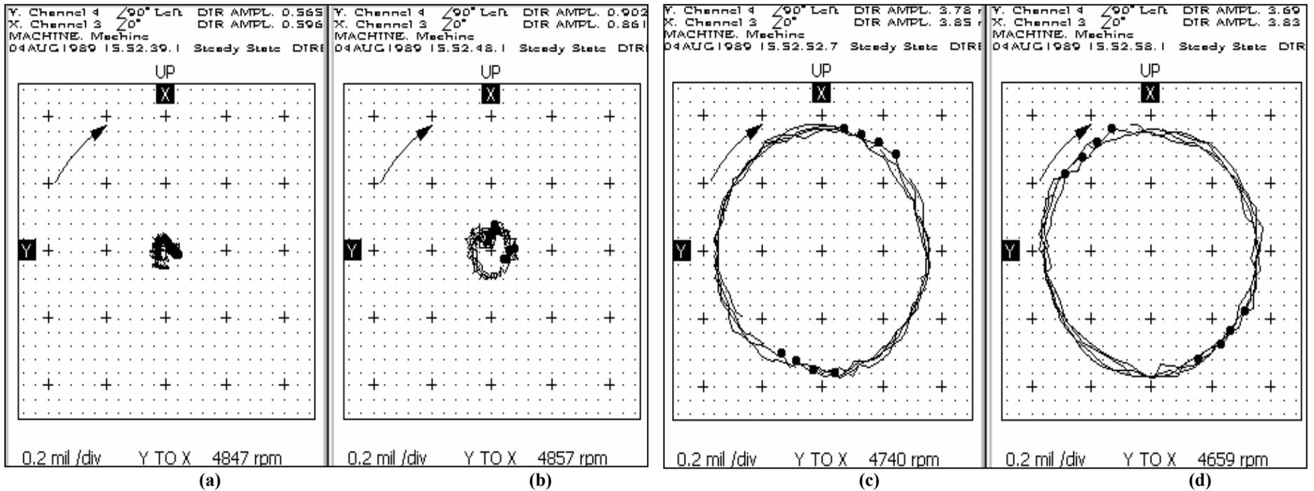
Figure 6.2 (a)-(d): The orbits illustrate the transition of rotor #1 to oil whirl instability. (September 2002).
