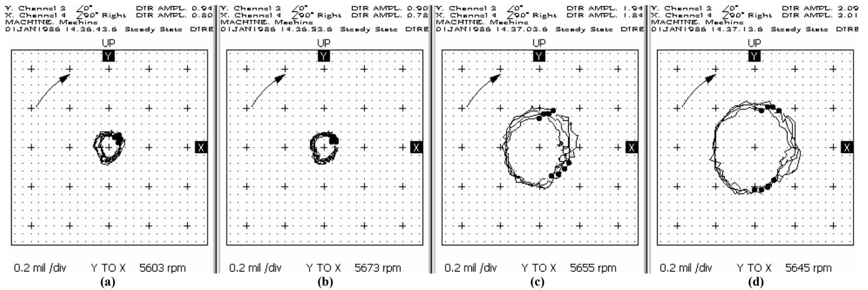
**Figure 6.4: The orbits illustrate the transition of rotor #1 to oil whirl instability. (February 2003).**
