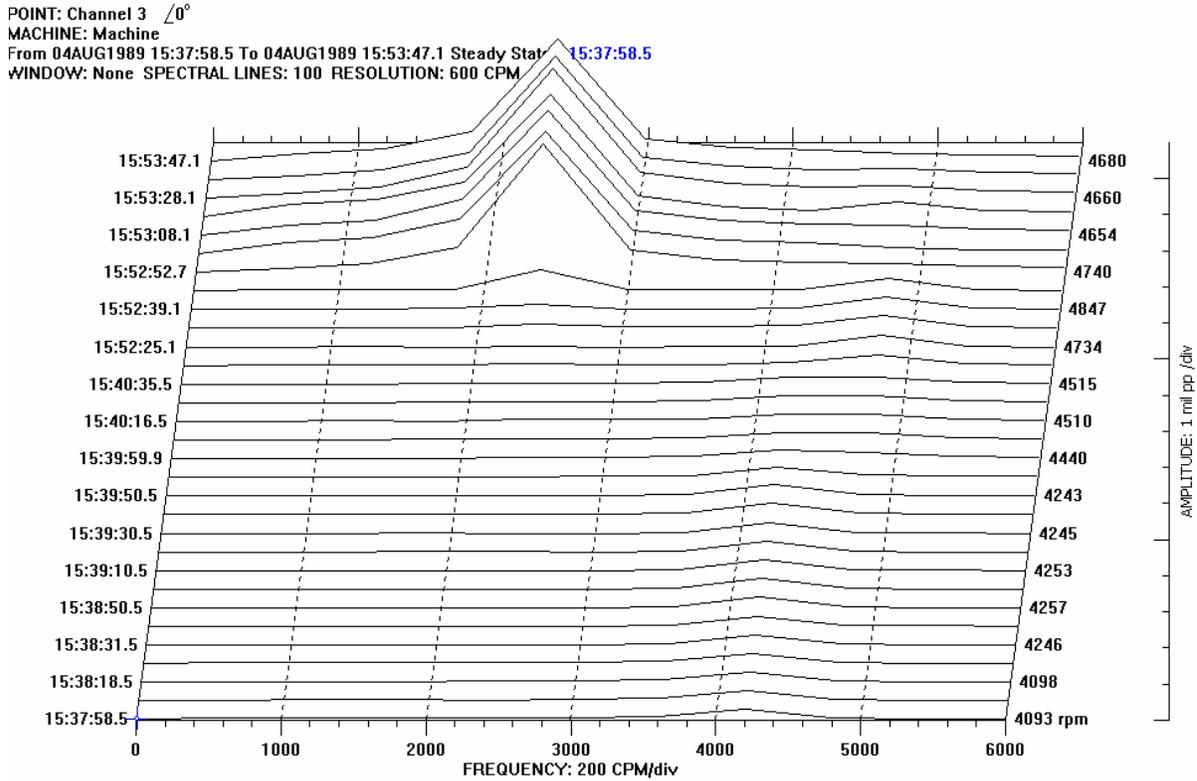
**Figure 6. 1: The waterfall plot of the experimental threshold of instability of rotor #1 (September 2002).**
