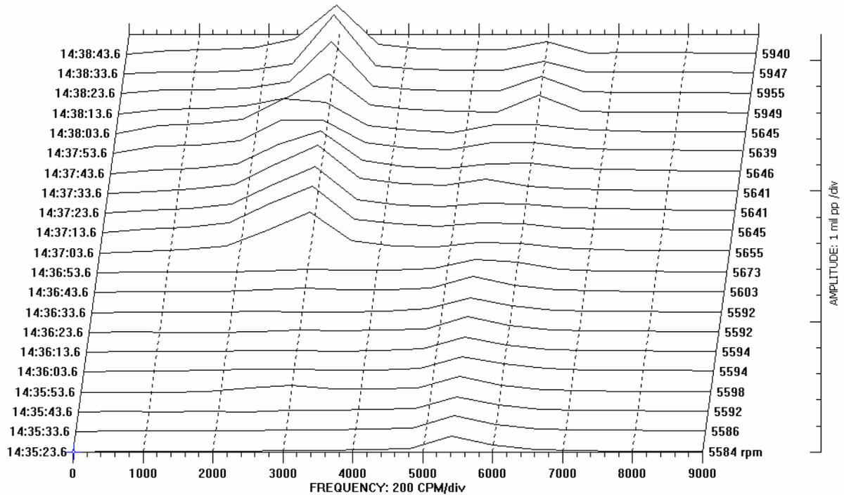
**Figure 6.3: The waterfall plot of the experimental threshold of instability of rotor #1 (February 2003).**
