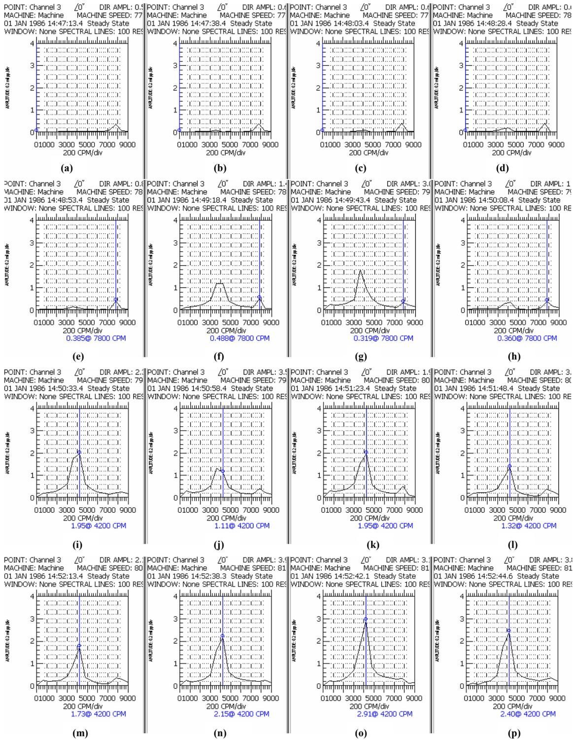
Figure 6.13 (a)–(p): The sequential spectrum plots of rotor #4 during oil supply temperature increase.
