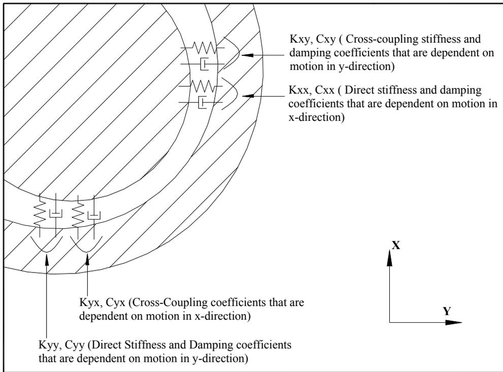
**Figure 2.2 Illustration of the eight dynamic coefficients of stiffness and damping**
