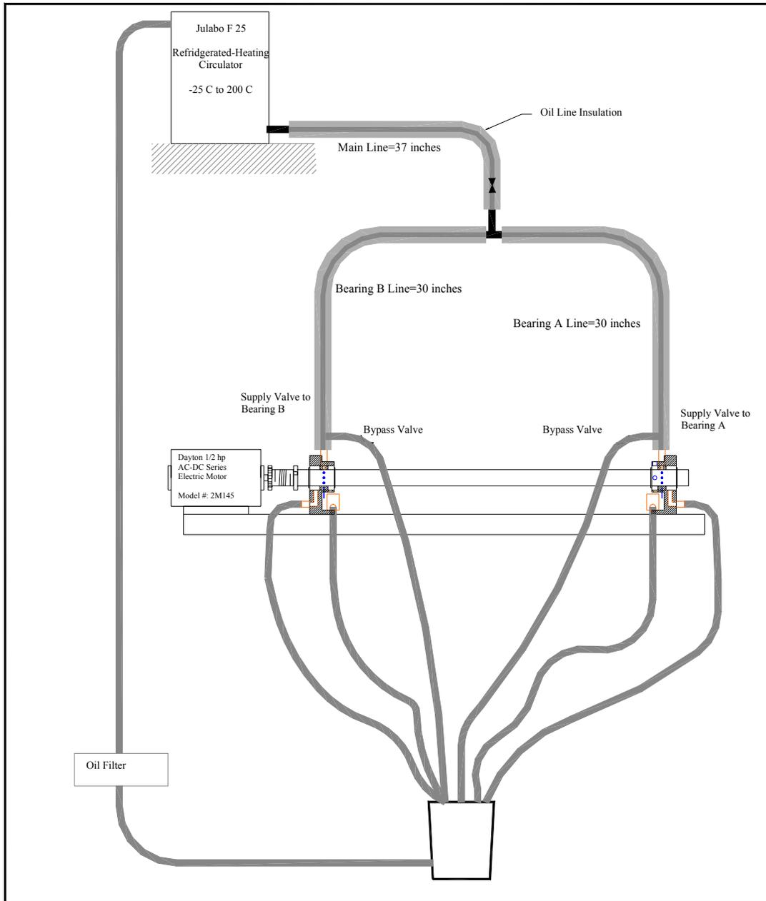
**Figure 5.1 is a general diagram of the oil supply to the bearings**
