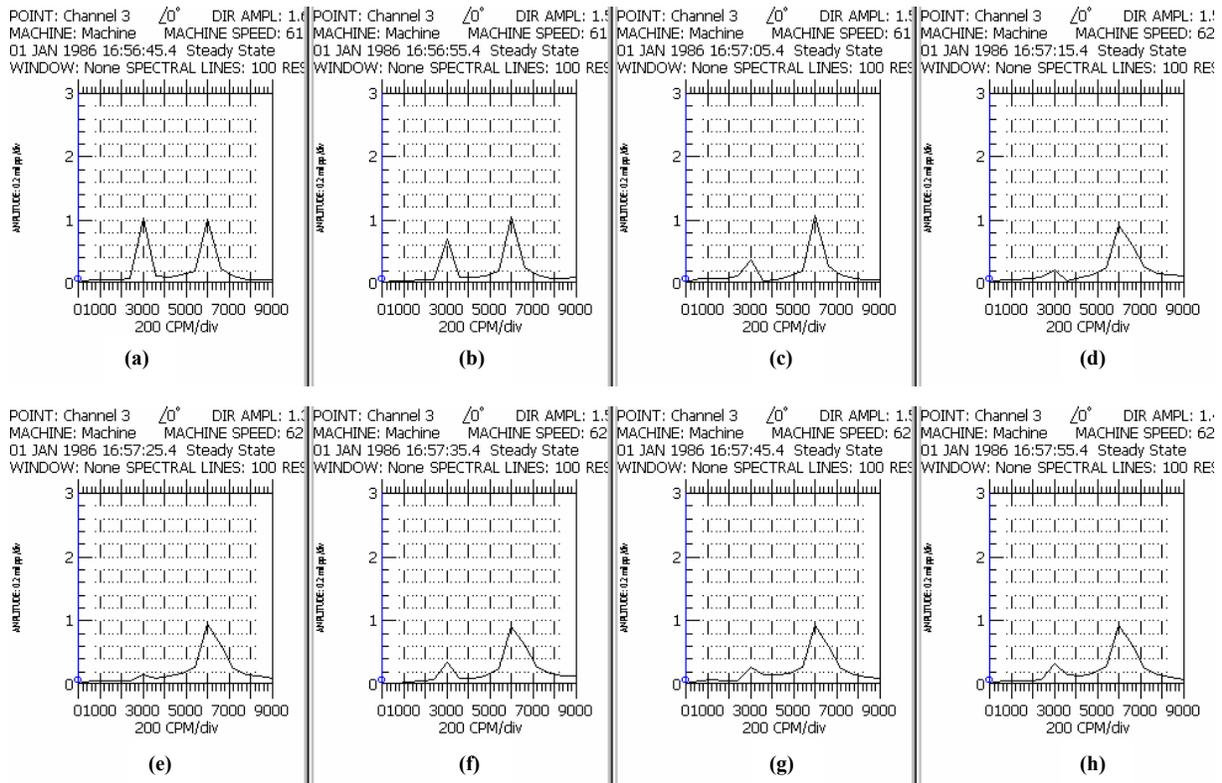
Figure 6.22(a)-(h): The spectrum plots for rotor #1 showing reluctance to whirl
