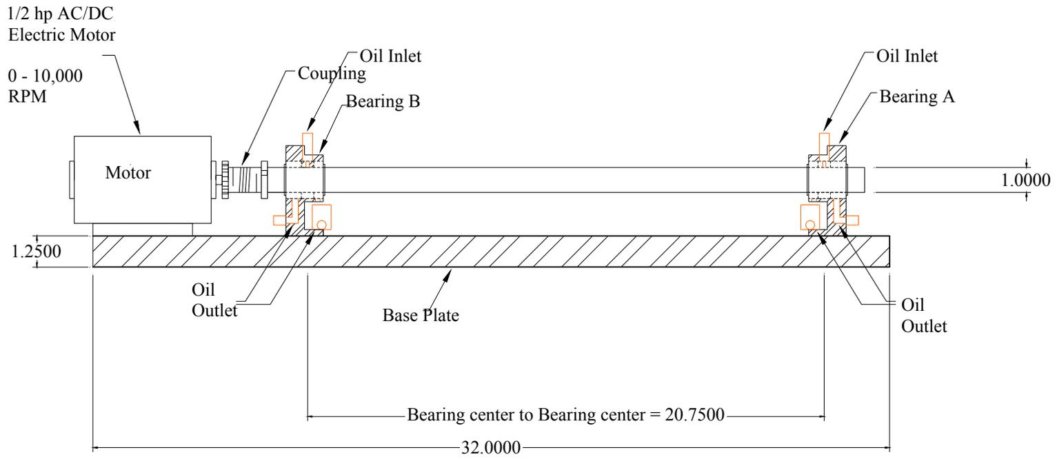
**Figure 4.1 Illustration of the experimental test rig**
