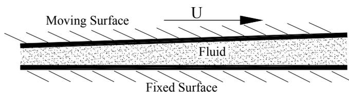
**Figure 3.1 is the basic geometry of any hydrodynamic lubrication**
