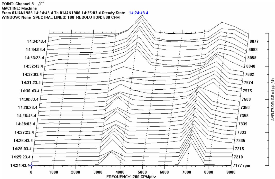
**Figure 6.19: The waterfall plot of rotor #3 after re-balancing.**
