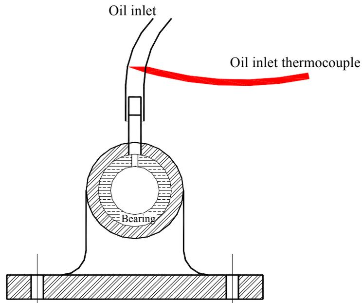
**Figure 4.6 Location of the inlet oil temperature measurement**
