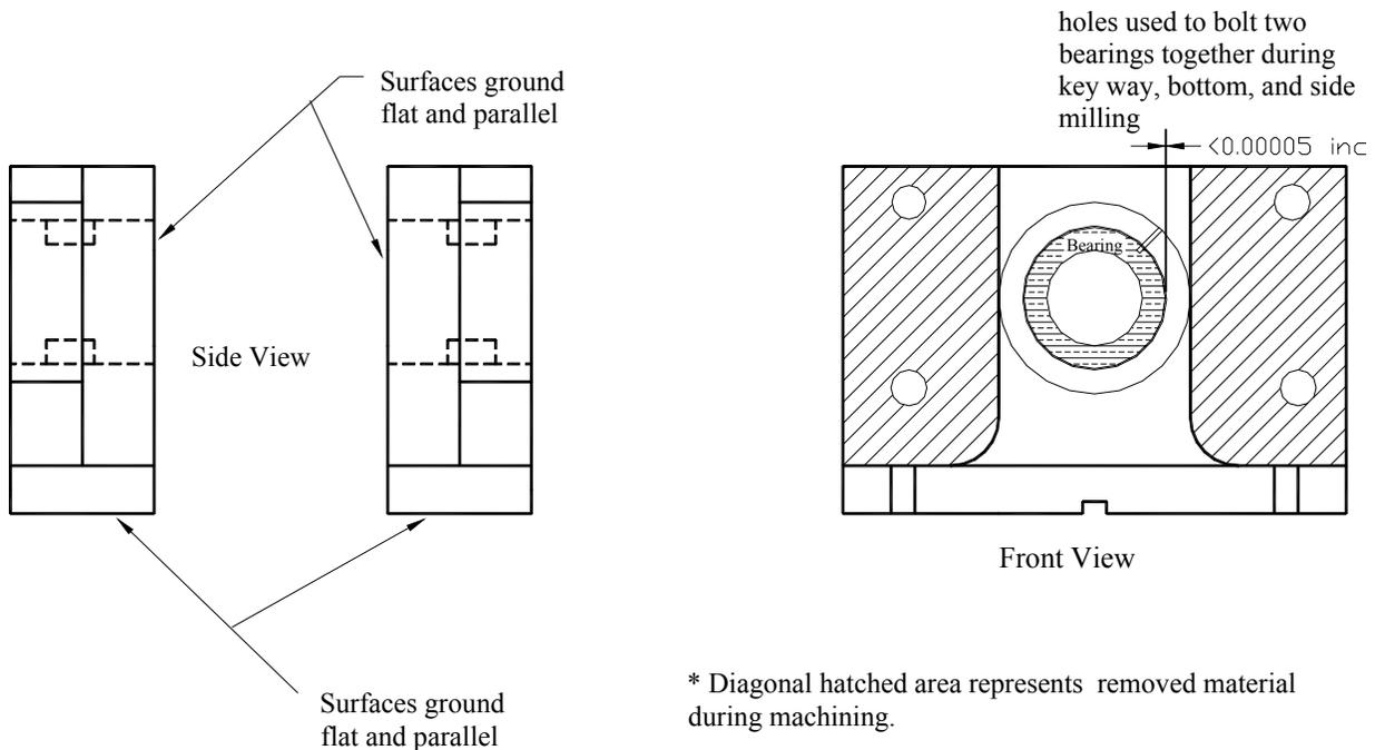
**Figure 4.3: Bearing housing as it is made from two blocks of steel**
