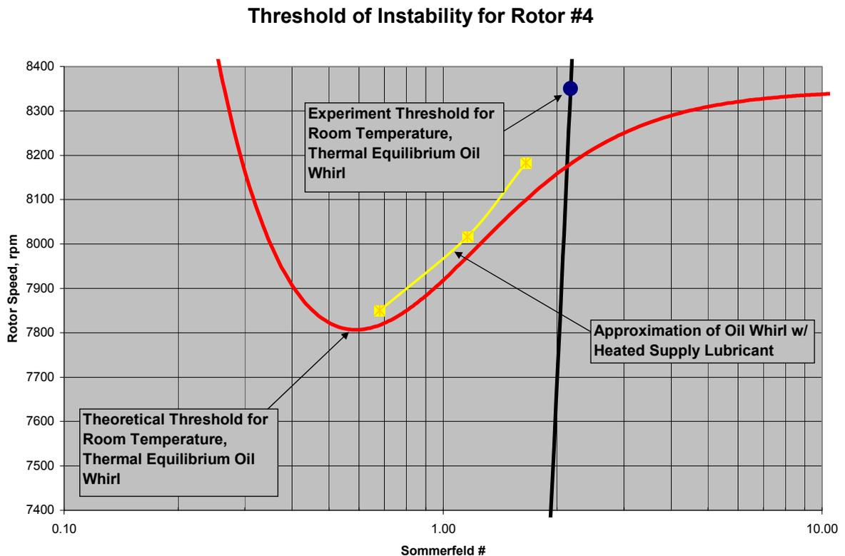
**Figure 7.1: Threshold of instability of rotor #4.**
