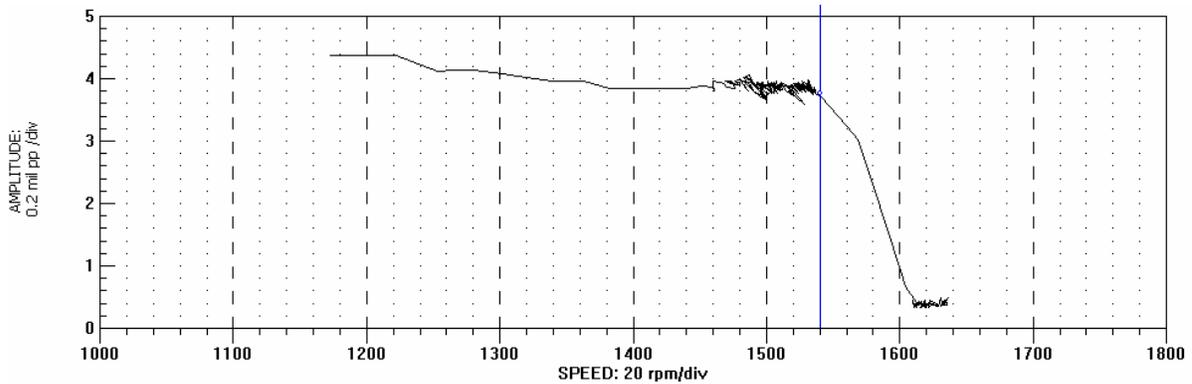
**Figure 6.5: The bode plot shows the initial high amplitude at start-up.**
