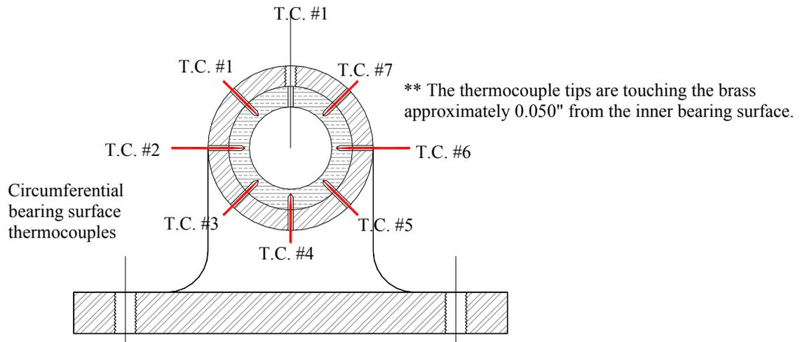
Figure 4.7 Circumferential position of the bearing temperature sensors
