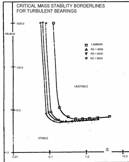
**Figure 2.8(c) Effect of turbulence on the whirl threshold [Craighead et al.]**
