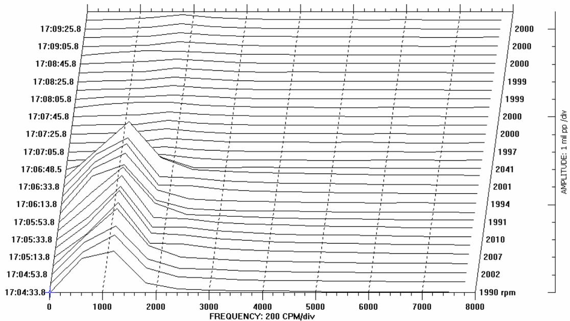
**Figure 6.6: The waterfall plot illustrates the initial occurrence of oil whirl**
