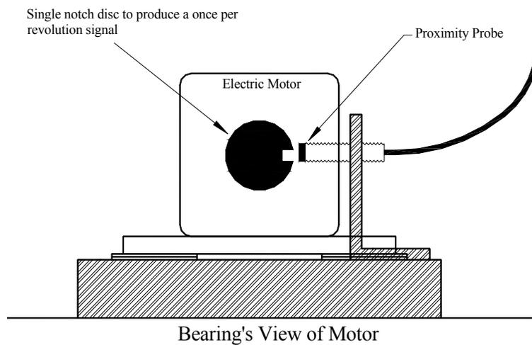
Figure 4.8 Proximity probe that marks the rotational speed (a once per revolution signal)
