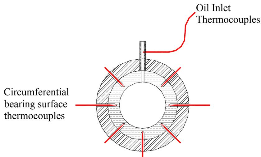
**Figure 2.6 Thermocouple locations for the inlet oil and the bearing surface**
