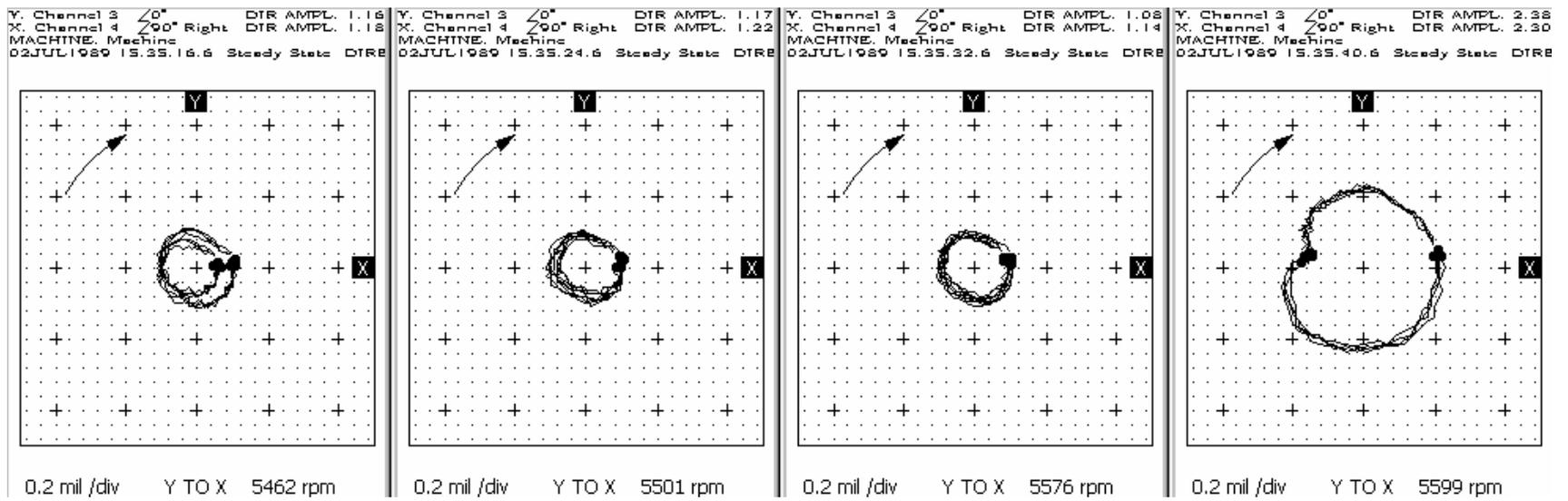
**Figure 6.16: The orbit of rotor #3 just after the damage occurred**
