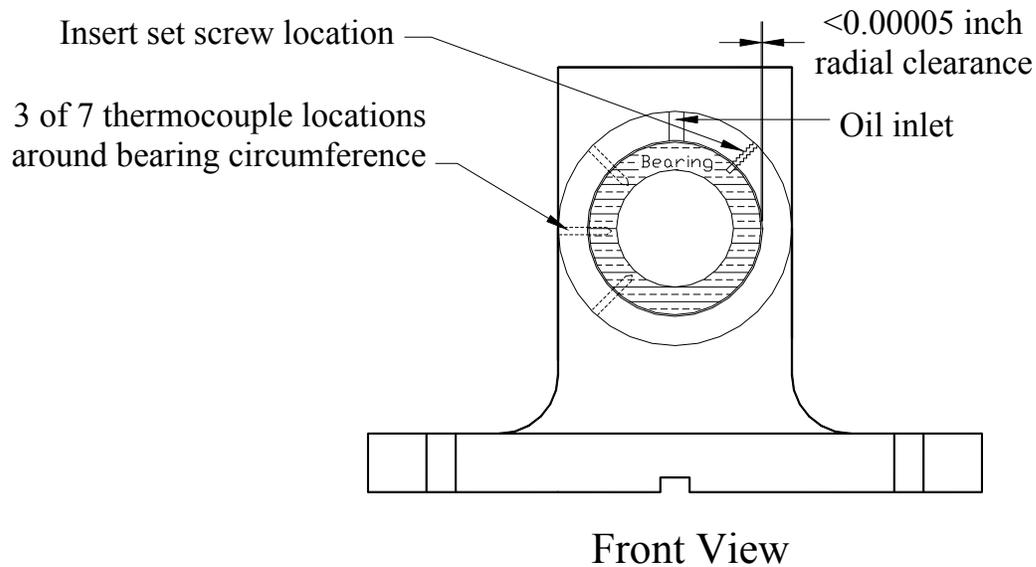
**Figure 4.4 Clearance between the bearing and the bearing housing**
