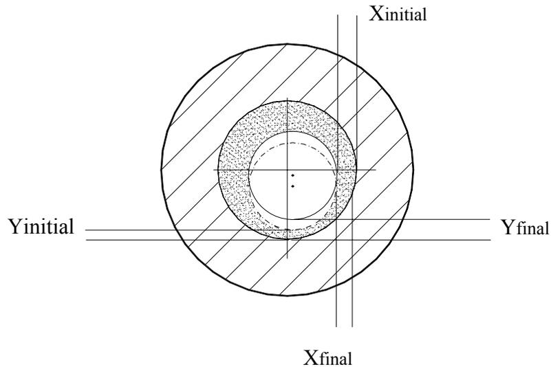
**Figure 2.1 Effect of shaft movement in purely the y-direction with the resulting change in film thickness in the x-direction**
