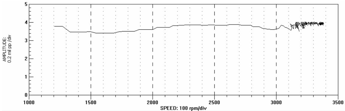
**Figure 6.8: The bode plot illustrating a non-stabilizing, oil whirl start-up.**
