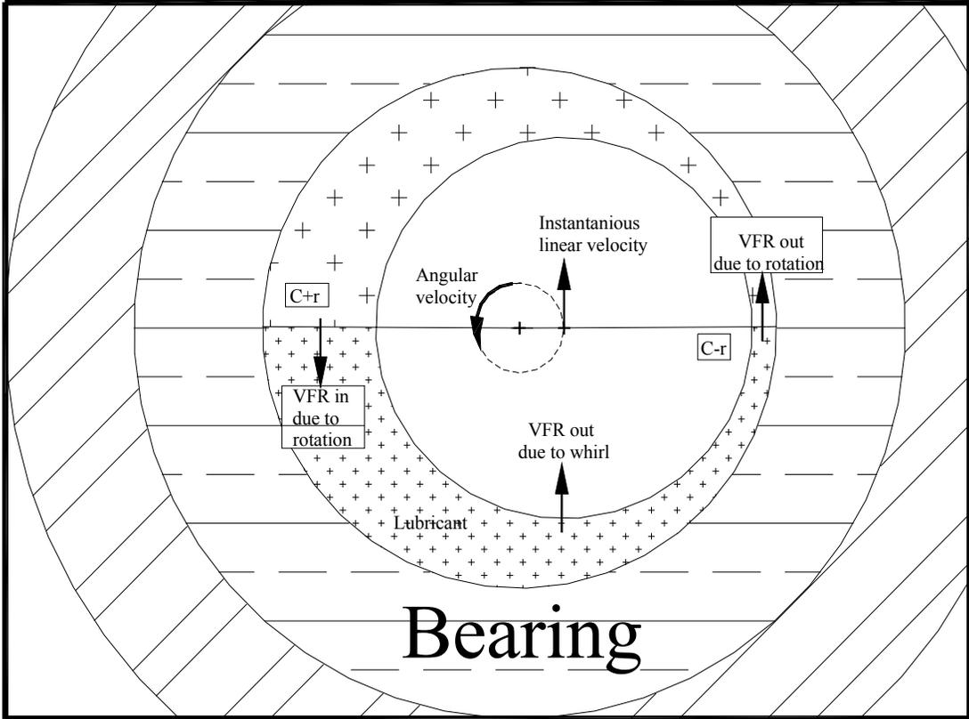
**Figure A.1: Control volume of lubrication film**
