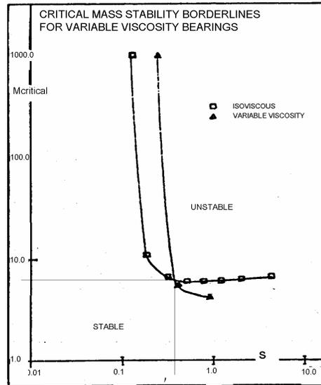
Figure 2.8(a) Effect of variable viscosity on the whirl threshold [Craighead et al.]
