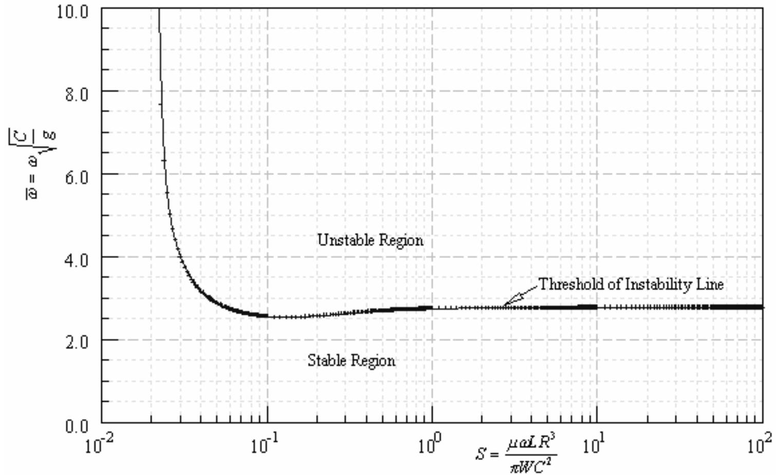
Figure 3.4 Threshold of whirl instability predicted by linear theory
