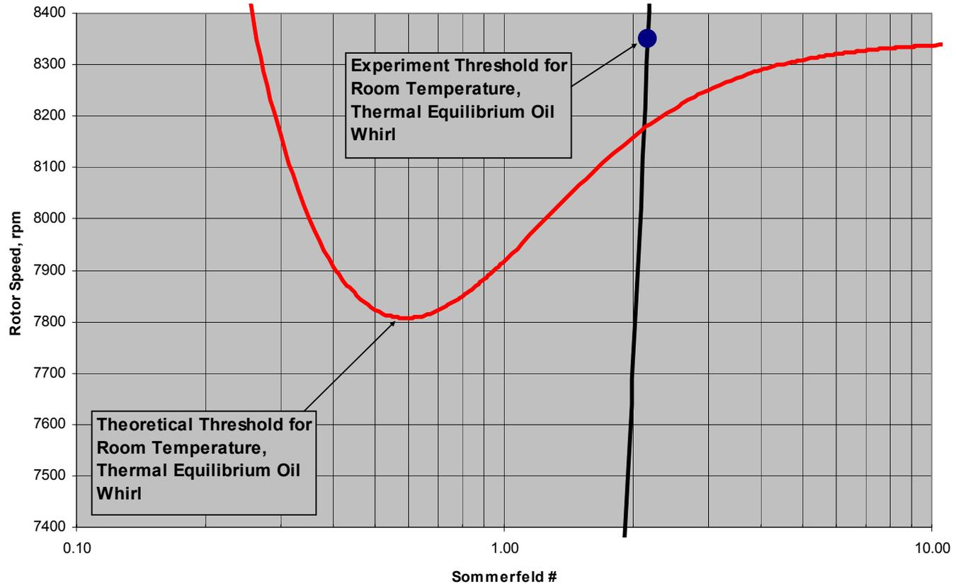
Figure 6.14 Theoretical threshold of instability illustrating “dip”
