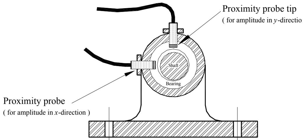
**Figure 4.9 Proximity probes used to measure the vibration amplitude**
