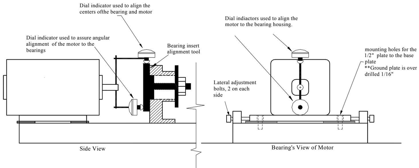
**Figure 4.5 Basic diagram of the motor alignment tools and their functions**
