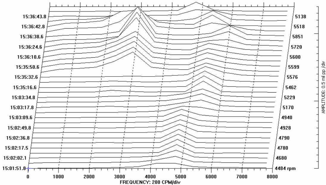
**Figure 6.17: The waterfall plot of rotor #3 after the damage occurred.**
