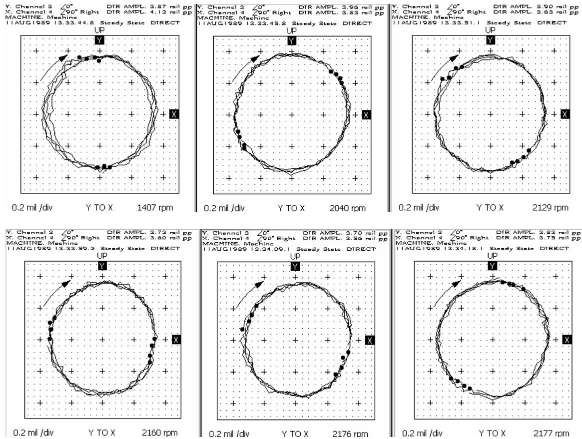
Figure 6.7: The orbit plots of initial oil whirl that does not cease.
