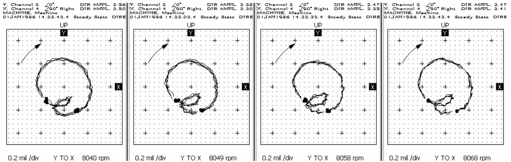
**Figure 6.18: Orbits of rotor #3 after damage and rebalancing**
