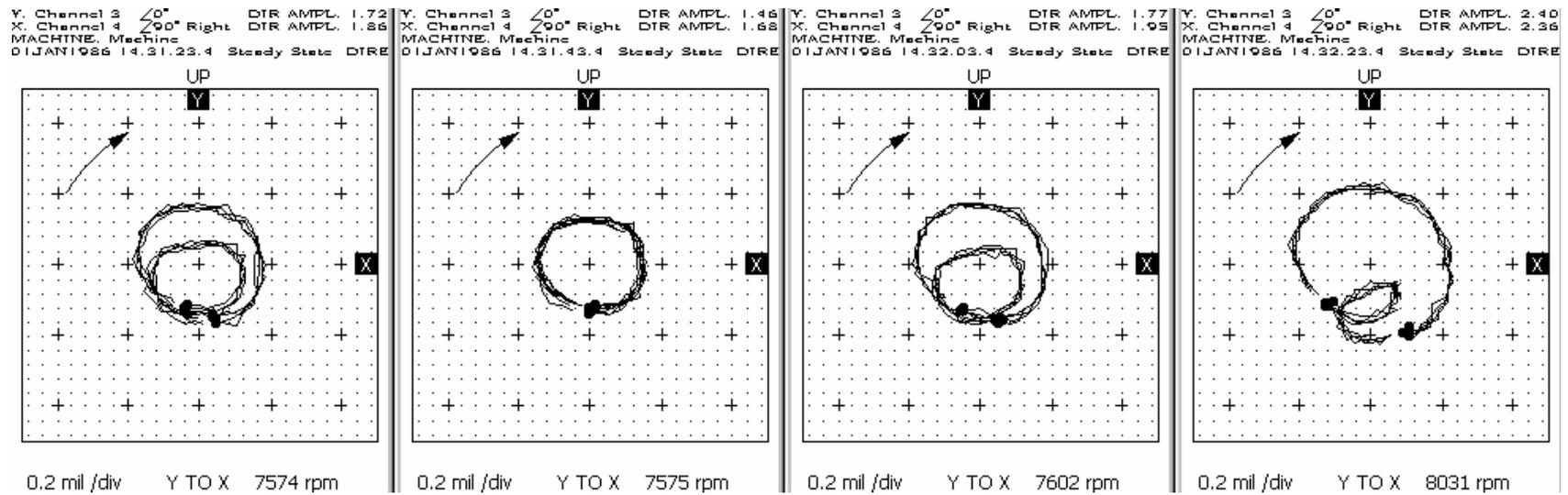
Figure 6.20: Orbit of rotor #3 after re-balancing
