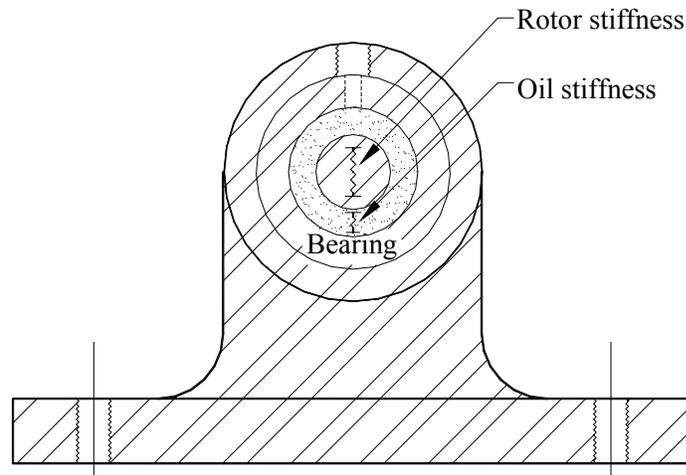
**Figure 2.3 Illustration of uni-direction stiffness in the rotor bearing system**
