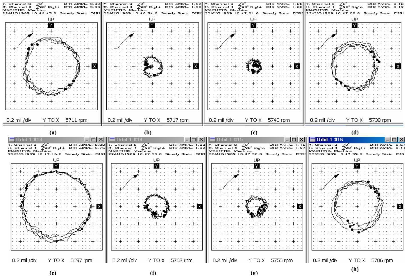
Figure 6.21(a)-(h): Orbits of rotor #3 not maintaining whirl
