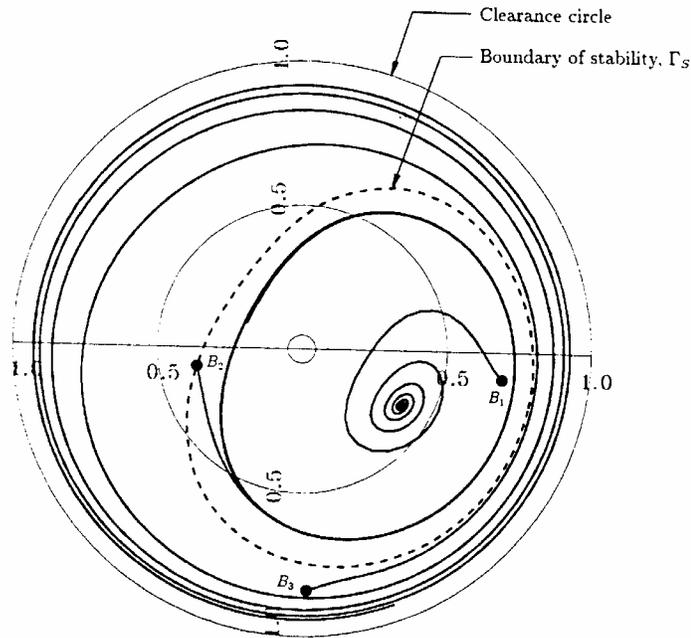
**Figure 2.9 Illustration of the stability boundary with a journal bearing clearance circle. [Khonsari and Chang]**
