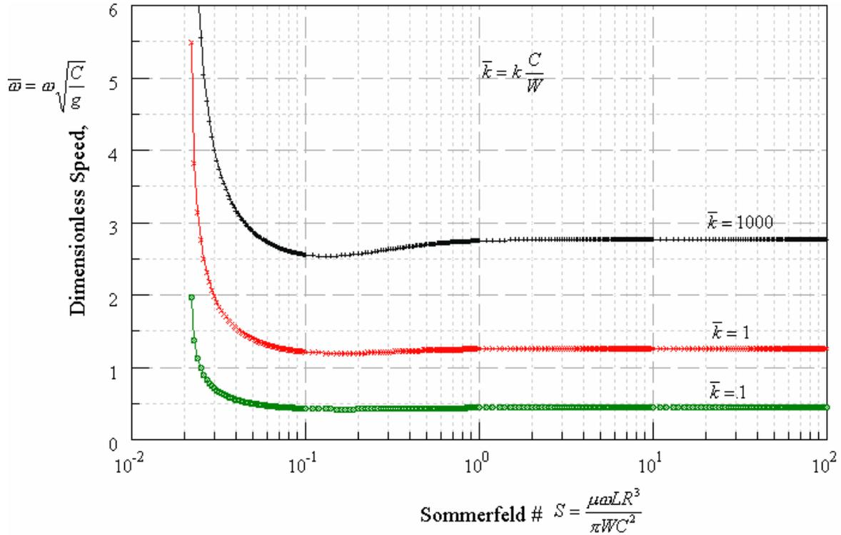
**Figure 2.5 Effect of rotor stiffness on oil whirl stability**
