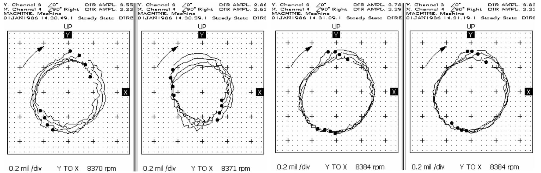
**Figure 6.11: The orbit of rotor #4 just beyond the threshold of instability**
