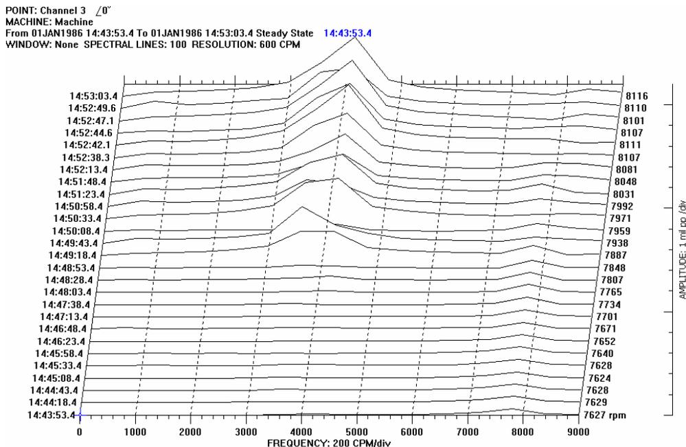
**Figure 6.12: The waterfall plot of rotor #4 as it approaches the threshold via increase in oil temperature**
