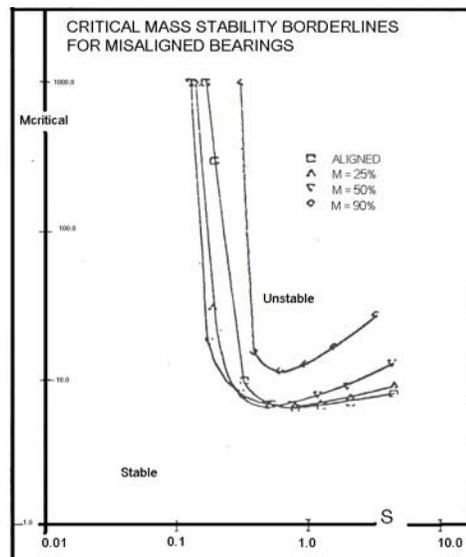
Figure 2.8(b) Effect of misalignment on the whirl threshold [Craighead et al.]
