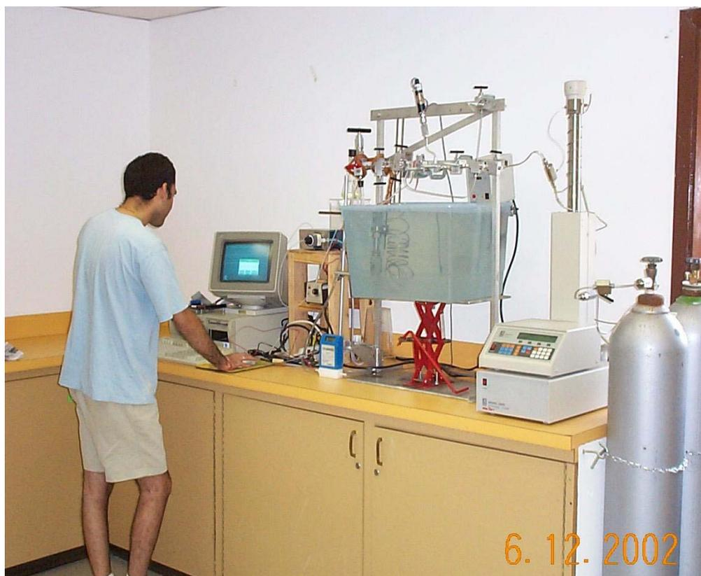
Figure 3.3. Laboratory scale SFE unit used in present study
