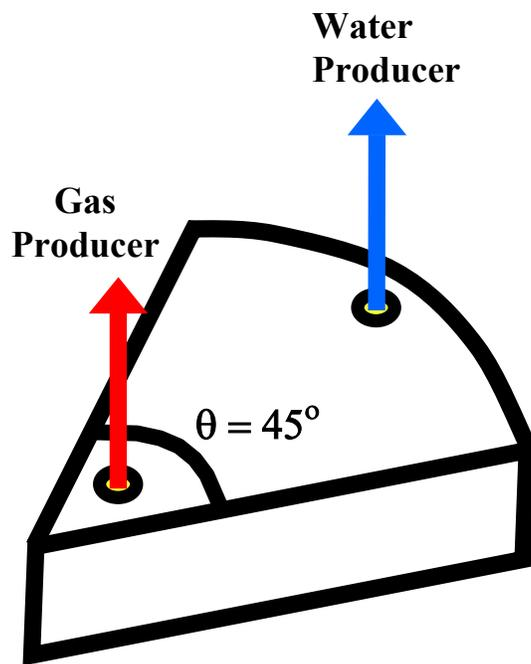
**Figure 4.1** Coproduction simulation model diagram.
