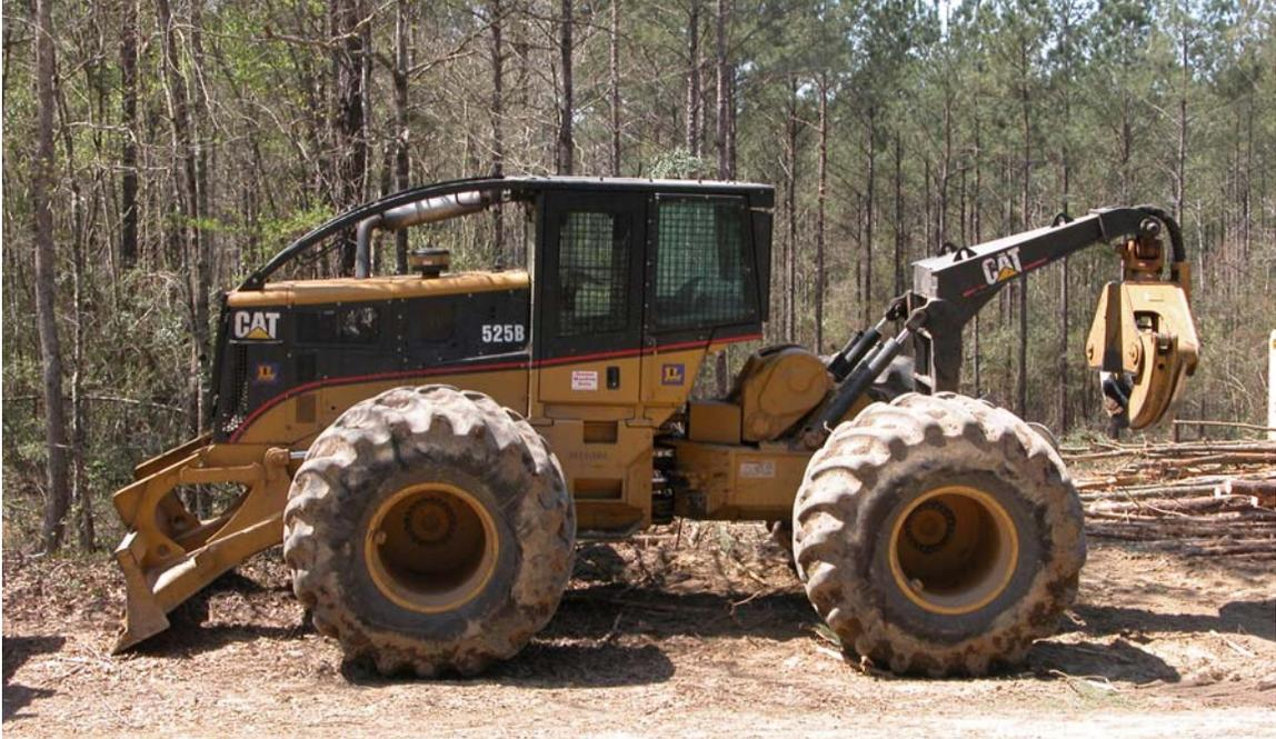
**Figure 1.** Picture of a Cat 525B Rubber-Tired Grapple Skidder.
