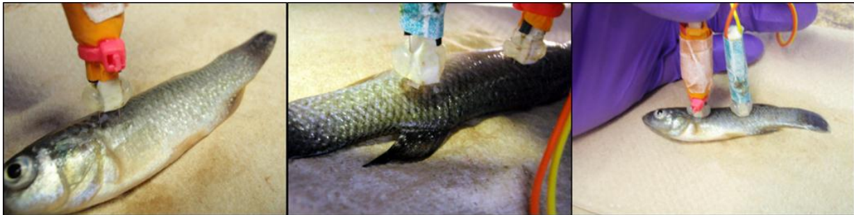
Figure 1. Photos showing positioning of probes for bioelectrical impedance analysis on F. grandis . Positive probe is lined up near base pectoral fin even with the top of the operculum, and negative probe was lined up with the front edge of the dorsal fin and the top of the operculum
