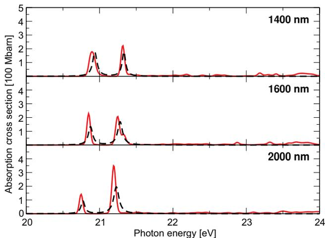
FIG. 4: (Color online) Laser-dressed XUV absorption cross section of helium for 1400, 1600, and 2000 nm laser wavelengths at a laser intensity of  $10^{12} \frac{\text{W}}{\text{cm}^2}$  (red solid curves). The results of the simple three-level model of Fig. 5 are indicated by the dashed black curves for  $\Gamma_{1s^{-1}2p} = 0.1 \text{ eV}$  and  $\Gamma_{1s^{-1}2s} = 0.05 \text{ eV}$ .
