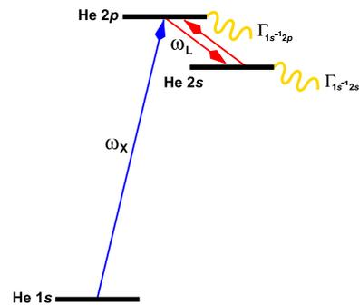
FIG. 5: (Color online)  $\Lambda$ -type three-level model for helium. The laser photon energy is  $\omega_L$  and the XUV photon energy is  $\omega_X$ . The laser-induced decay widths of the  $1s^{-1}2p$  and  $1s^{-1}2s$  excited states are denoted by  $\Gamma_{1s^{-1}2p}$  and  $\Gamma_{1s^{-1}2s}$ , respectively.
