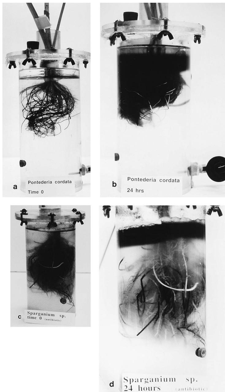
FIG. 7. Pattern of root oxidation of methylene blue in whole-plant chambers with intact sediment-free roots of *P. cordata* at 0 h (a), *P. cordata* at 24 h (b), *S. eurycarpum* at 0 h (c), and *S. eurycarpum* at 24 h (d).
