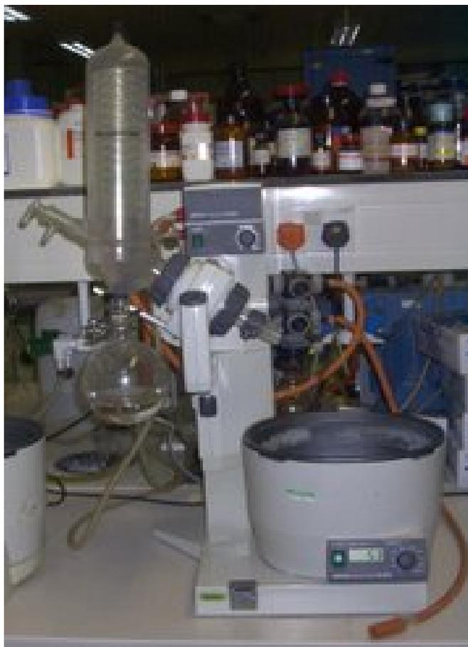
Figure 2-1. Picture of the rotary evaporator.
