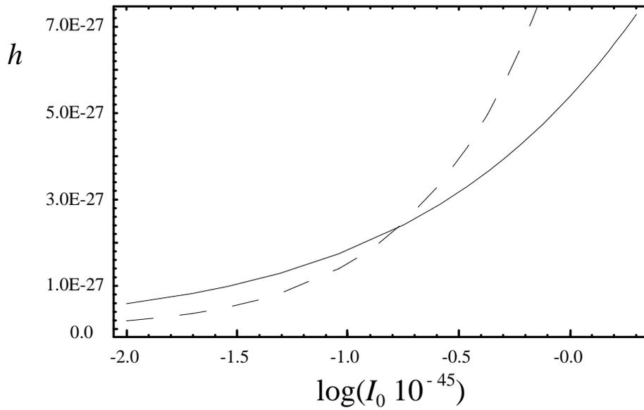
Fig. 4.— The amplitude of the strain at the Earth given by equation (18) – leaving out dependences on  $i$  and  $t$  – as a function of the moment of inertia involved in the precession, in units of  $10^{45}$  g cm<sup>2</sup>. The dashed curve corresponds to the contribution from the  $\omega$  term and the solid curve to the  $2\omega$  term.
