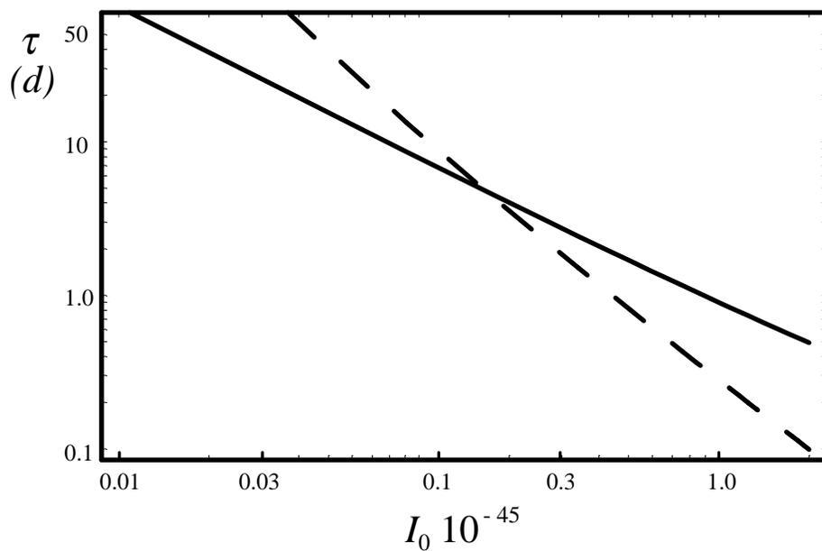
Fig. 6.— Estimated integration times for a 4 sigma detection by LIGO II for the signal at  $\omega$  (dashed) and at  $2\omega$  (solid) as a function of  $I_0$  in units of  $10^{45}$  g cm<sup>2</sup>. The curves shown above have been estimated using the minimum strain level for an optimized LIGO II,  $h_d = 1.5 \times 10^{-24}$ . For higher noise levels, the integration times scale as  $(h_d/1.5 \times 10^{-24})^2$ .
