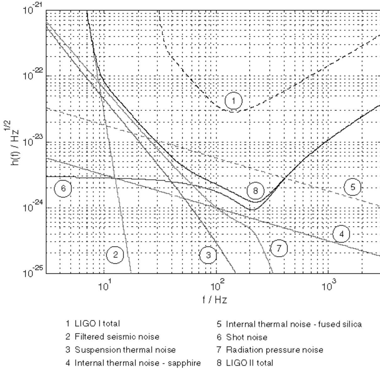
Fig. 5.— Preliminary estimates of the noise spectrum expected for LIGO II. The contributions from various sources are shown separately and added together (See <http://www.ligo.caltech.edu/docs/M/M990288-A1.pdf>).
