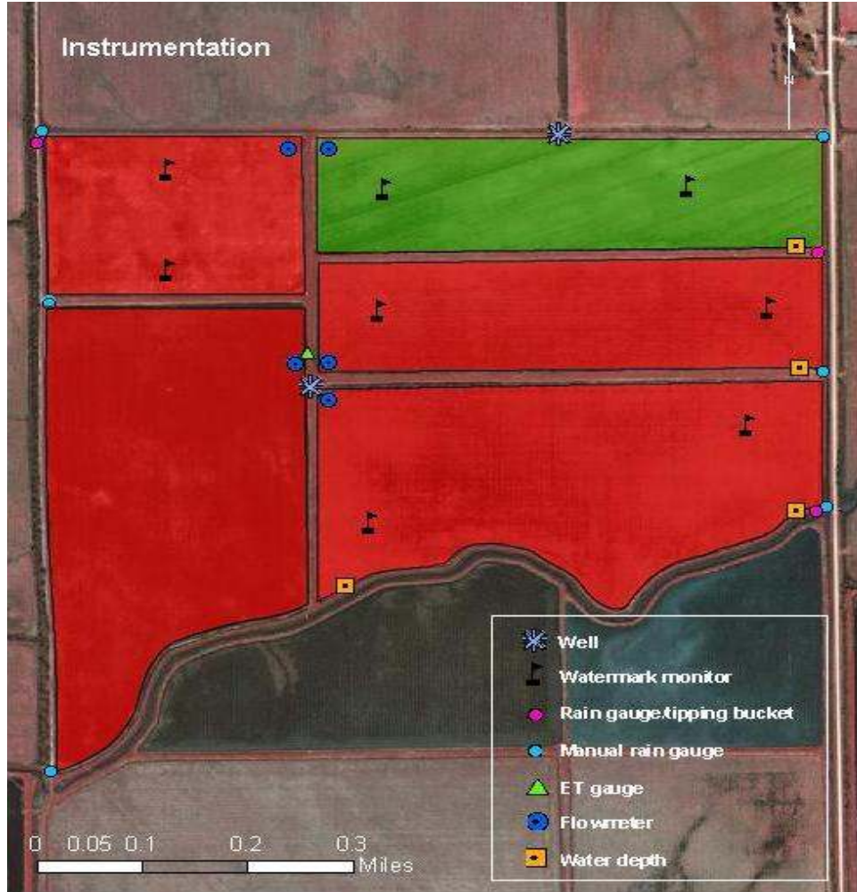
Figure A.1. Instrumentation layout for fields 2-8, 2-9, 2-10, 2-11, and 2-12 (western fields 2006). Level fields are in red and the sloped one in green.
