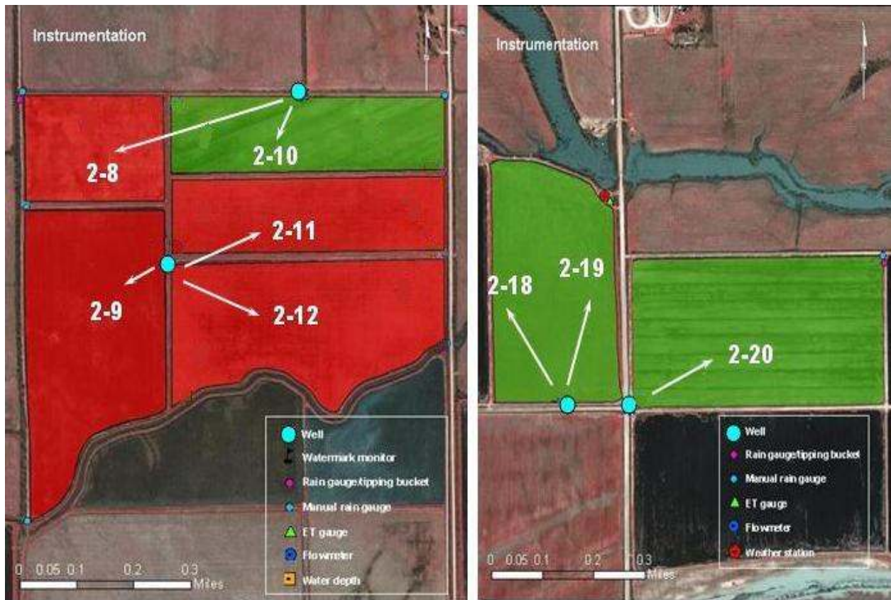
Figure A.7 Wells distribution and water allocation between fields at Angelina Plantation during 2006. Arrows indicate the fields served by each well.
