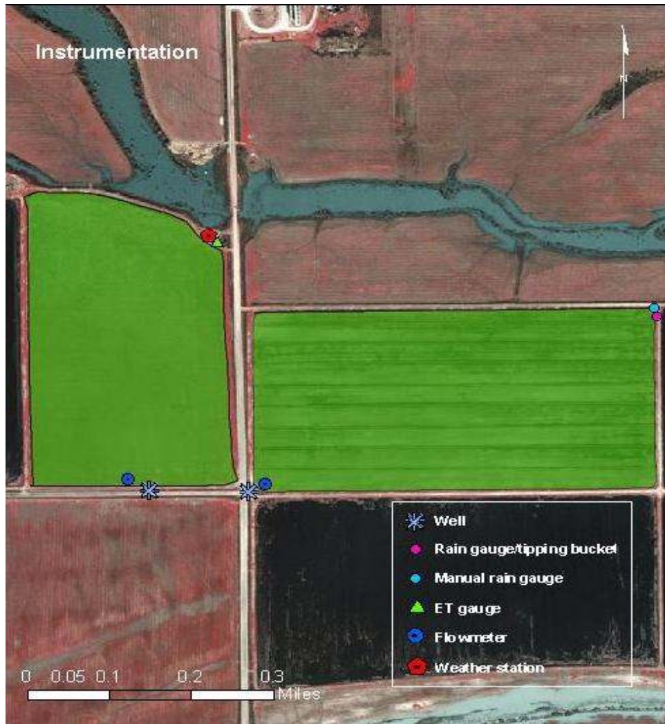
Figure A.2. Instrumentation layout for fields 2-19 and 2-20 (eastern fields 2006).
