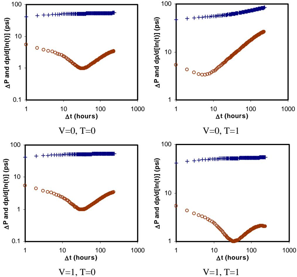
**Figure 8. Log-log plots for leaky-compartment model**
