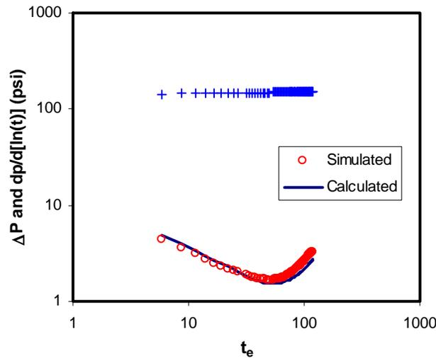
**Figure 37. Example of fitting derivative curve using response surface model**
