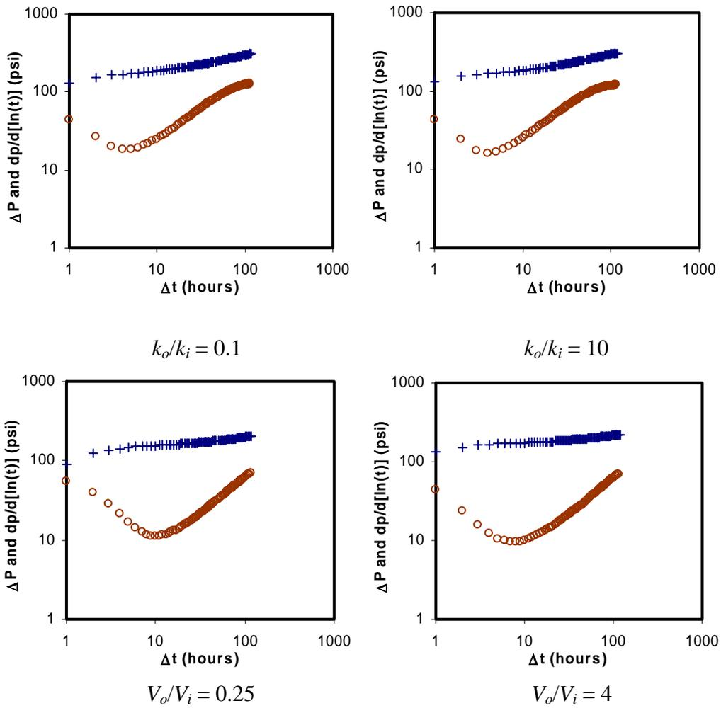
**Figure 36. log-log plot for the mixed model with different compartment property**
