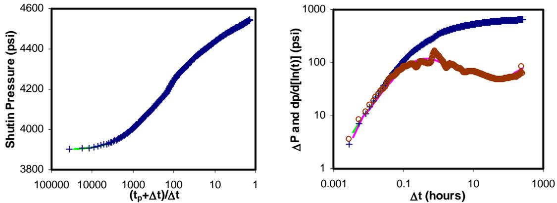
**Figure 3. Horner and log-log plot of Well A3 in Tahoe Field**
