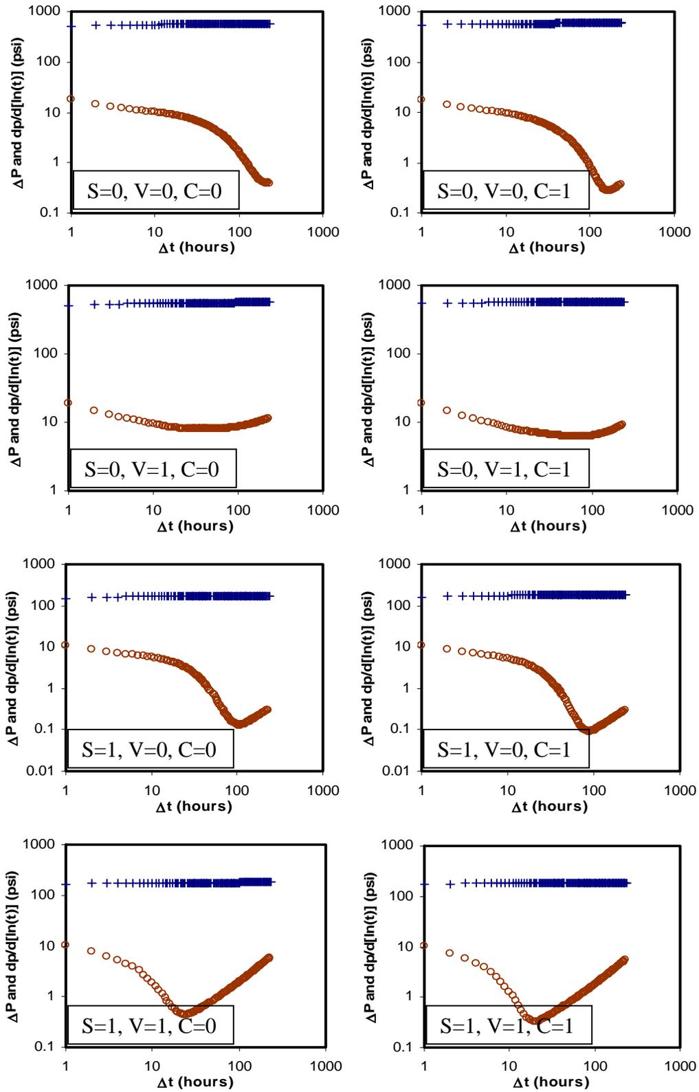
Figure 13. Log-log plots for the design for skin, pore volume and compaction
