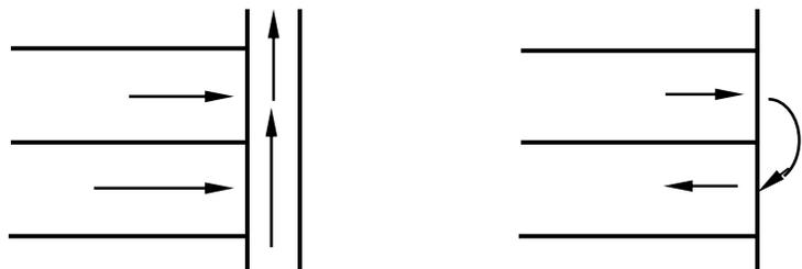
**Figure 15. Different flow profile for drawdown and buildup**
