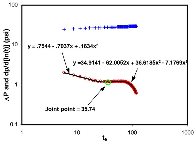
**Figure 29. Example 1 for Leaky-compartment model with piecewise regression**
