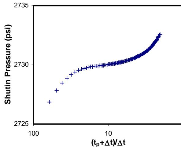
**Figure 14. Horner plot for the case of permeability in contrast to pore volume**
