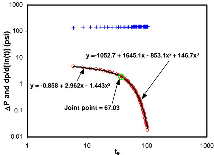
**Figure 26. Example 1 for crossflow system with piecewise regression**
