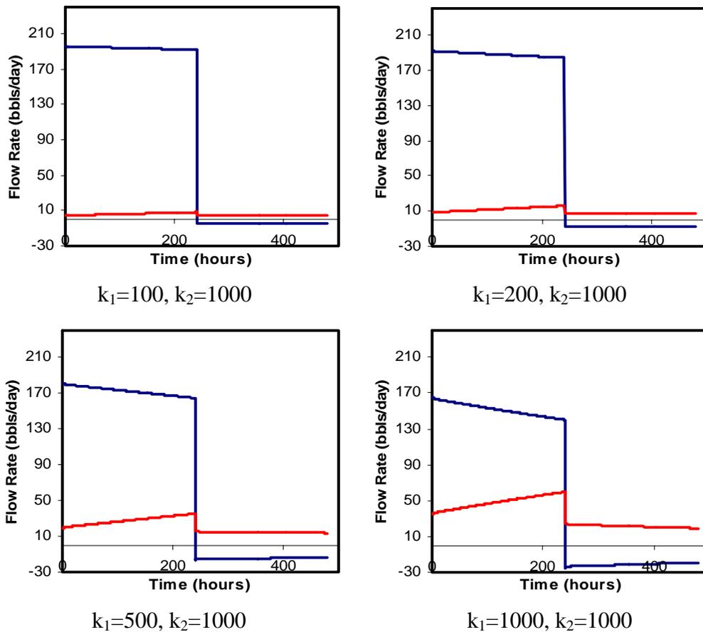
**Figure 20. Layer flow rates for varying first-layer permeability**
