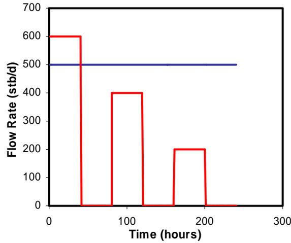
**Figure 32. Constant rate and variable rate used in the deconvolution**
