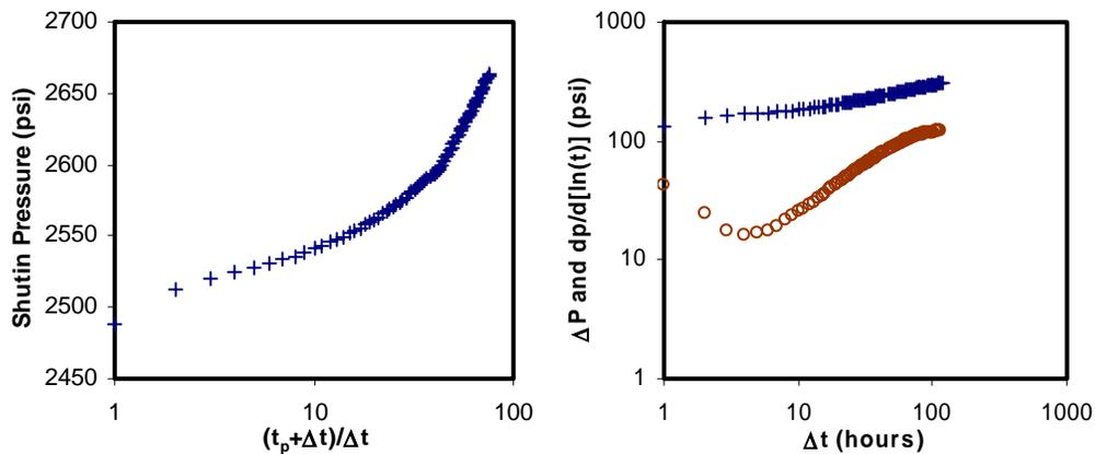
**Figure 35. Horner and log-log plot of the pure layered model**
