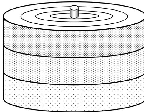
**Figure 21. Schematic graph of 3-layer radial model**
