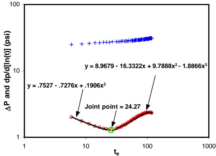
**Figure 30. Example 2 for Leaky-compartment model with piecewise regression**
