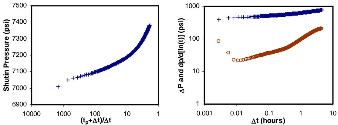
**Figure 2. Horner and log-log plot of Well A2 in Ram Powell Field**
