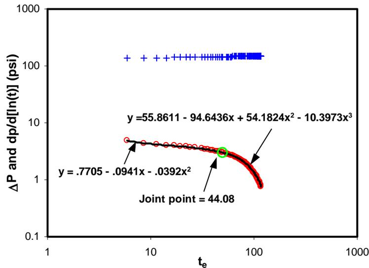
**Figure 27. Example 2 for crossflow system with piecewise regression**
