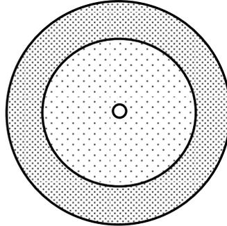
**Figure 7. Leaky compartments represented by a two-zone radial model**
