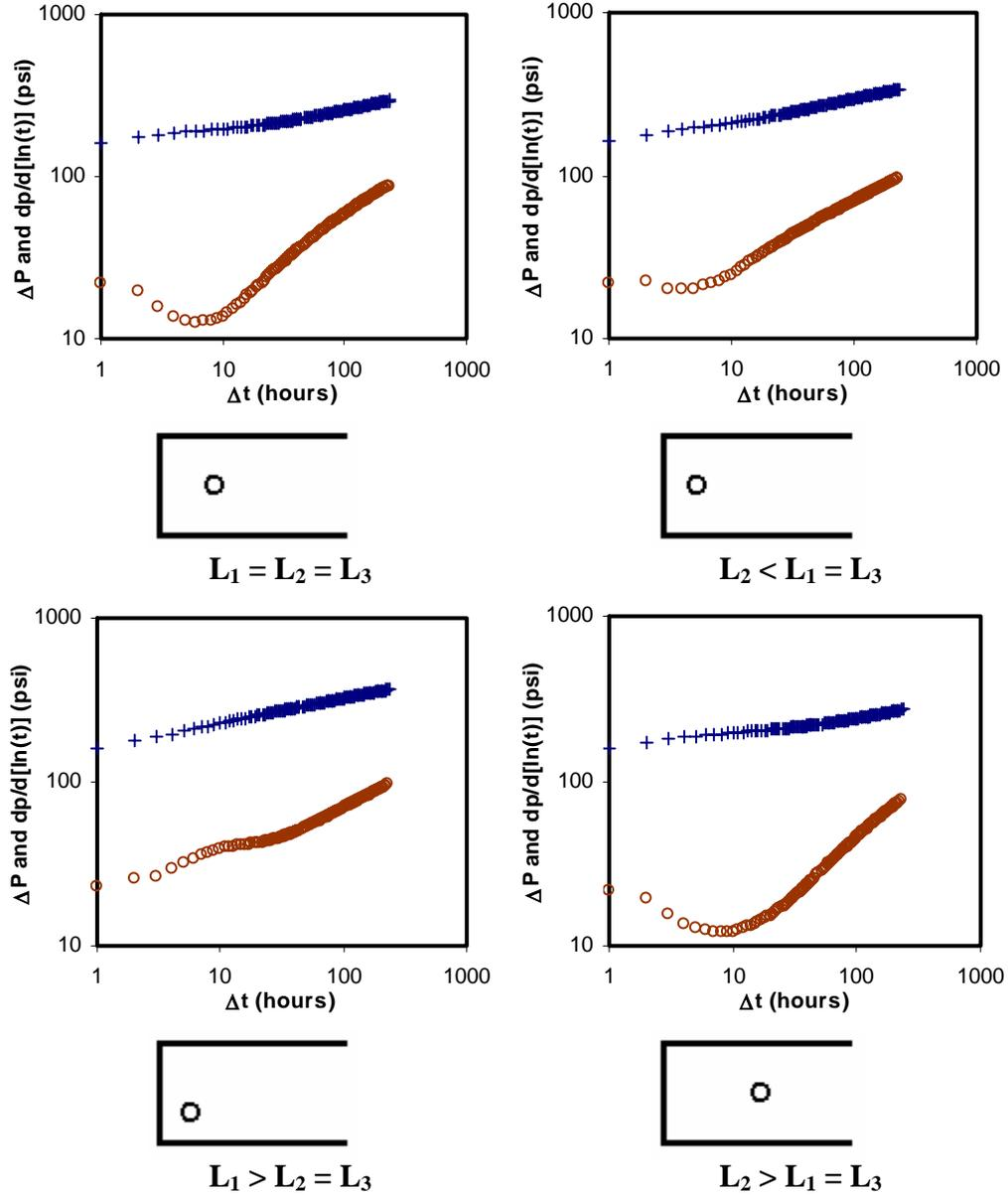
**Figure 6. Log-log plots for different well locations for U-shaped boundary model**
