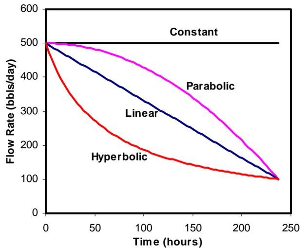
**Figure 9. Different types of variable flow rates**
