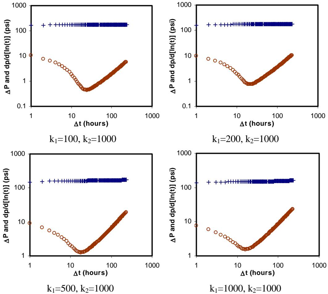
Figure 19. Log-log plots for varying first-layer permeability
