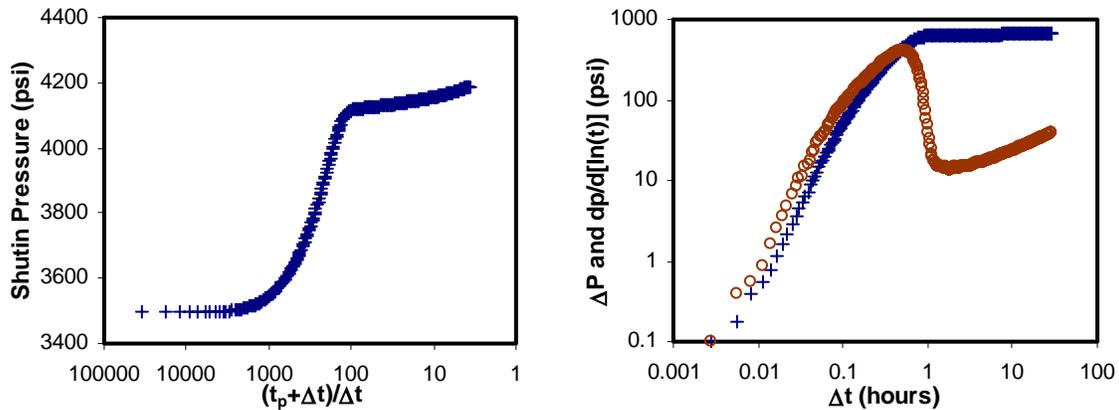
**Figure 4. Horner and log-log plot of Well SE in Tahoe Field**
