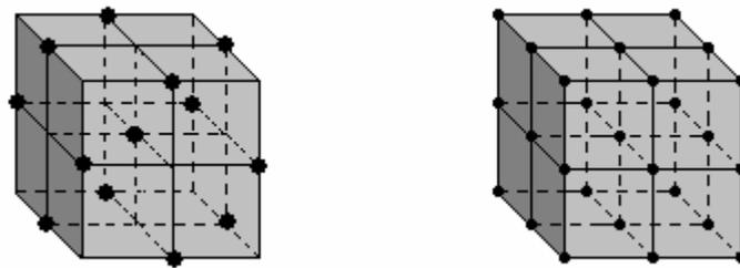
**Figure 22. Box-Behnken design and 3-level full factorial design**
