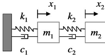
**Figure 2.1:** Simplified model of a two degrees-of-freedom system.
