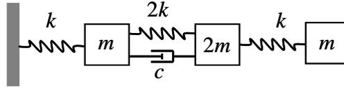
Figure 4.7: The open-loop system of Example 9.
