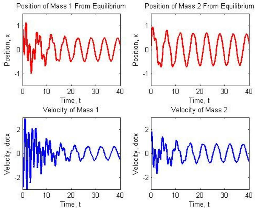
**Figure 2.3:** Simulation of example system displacement (top) and velocity (bottom), showing high frequency response stabilization from  $t=0-30$  and gradual decrease in amplitude of vibration for all  $t$ .
