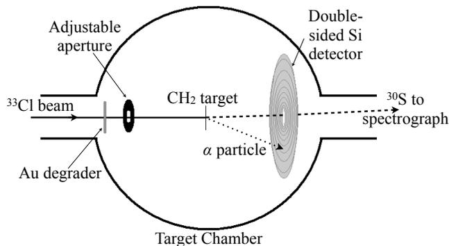
FIG. 2. A schematic of the experimental setup.
