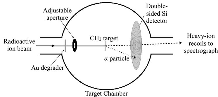
**Figure 1.** A schematic of the experimental setup.
