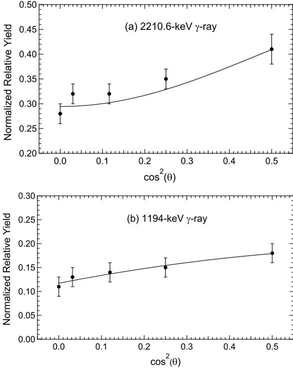
Figure 8: Experimental  $\gamma$ -ray angular distributions of the 2210.6-keV (a) and the 1194-keV (b) transitions. Both  $\gamma$ -rays are observed in the singles spectra obtained during phase II of the experiment. They correspond to the  $2_1^+ \rightarrow 0_1^+$  and  $2_2^+ \rightarrow 2_1^+$  transitions in  $^{30}\text{S}$ , respectively. The solid lines are best fits to Legendre polynomials.
