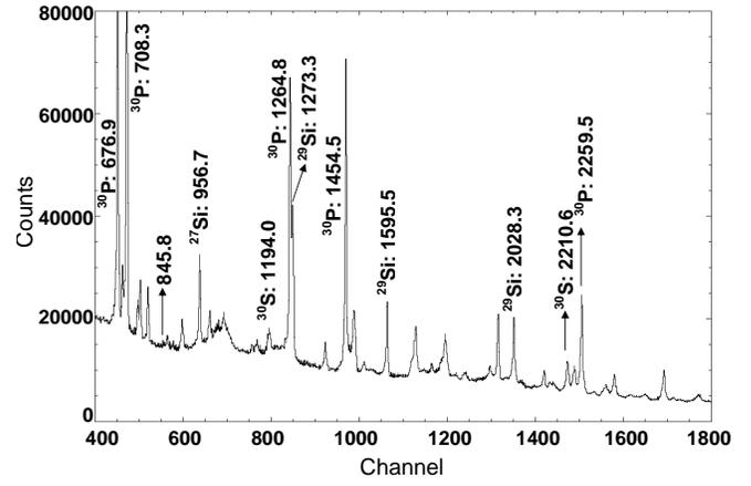
Figure 4: Singles  $\gamma$ -ray spectrum measured during phase II of the experiment at  $90^\circ$  using detector 1. Selected strong transitions are labeled by their parent nuclei and with energies (in keV) that are weighted averages between both phases of the experiment. The 2210.6-keV ( $2_1^+ \rightarrow 0_1^+$ ) and 1194-keV ( $2_2^+ \rightarrow 2_1^+$ ) peaks originate from levels in  $^{30}\text{S}$ .
