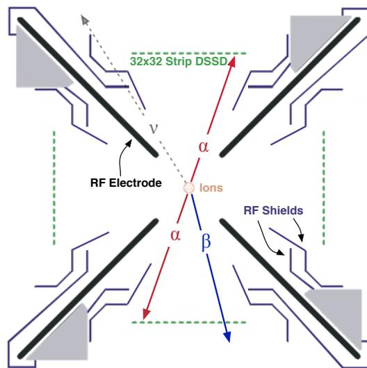
FIG. 1. Cross-sectional view of the BPT and detector system in the RF plane. The direction of the emitted  $\alpha$ s and  $\beta$ s is determined by the vector between the trap center and detector pixels.
