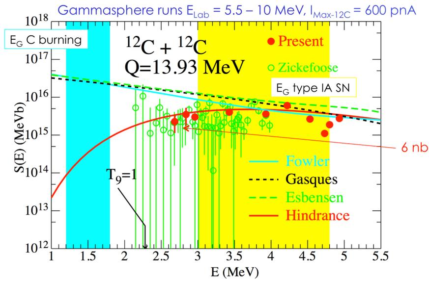
**Figure 3.** Red points :  $^{12}\text{C}+^{12}\text{C}$  S factors measured in this work. Green circles : results from ref. [12]. The blue, black, red and green dashed lines correspond to extrapolations from Fowler [13], Gasques [14], Jiang [15] and Esbensen [16].
