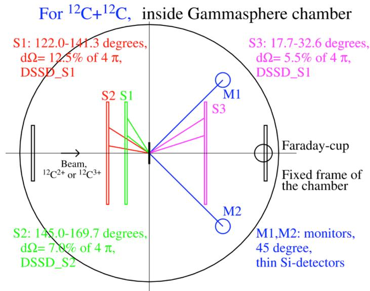
**Figure 2.** Schematic view of the target chamber showing the 3 annular DSSDs, the Si monitors and the Faraday cup.
