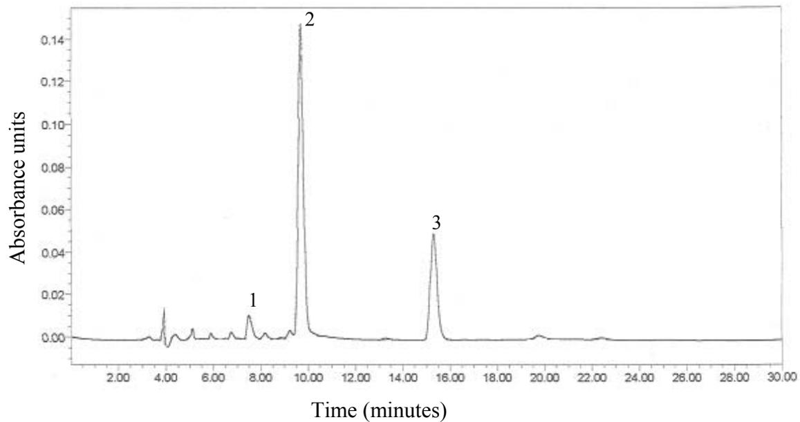
Figure 2.2. A representative chromatogram for a 20 µl sweetpotato extract analyzed with a Gemini C18, 5 µm, 4.6 × 250 mm column using a mobile phase consisting acetonitrile: 10 mM K<sub>2</sub>HPO<sub>4</sub> (20:80), pH 2.6; flow rate: 0.75 ml/min, temperature: 30 °C, UV detection at 320 nm. Peaks: (1) unknown, (2) chlorogenic acid, (3) caffeic acid.
