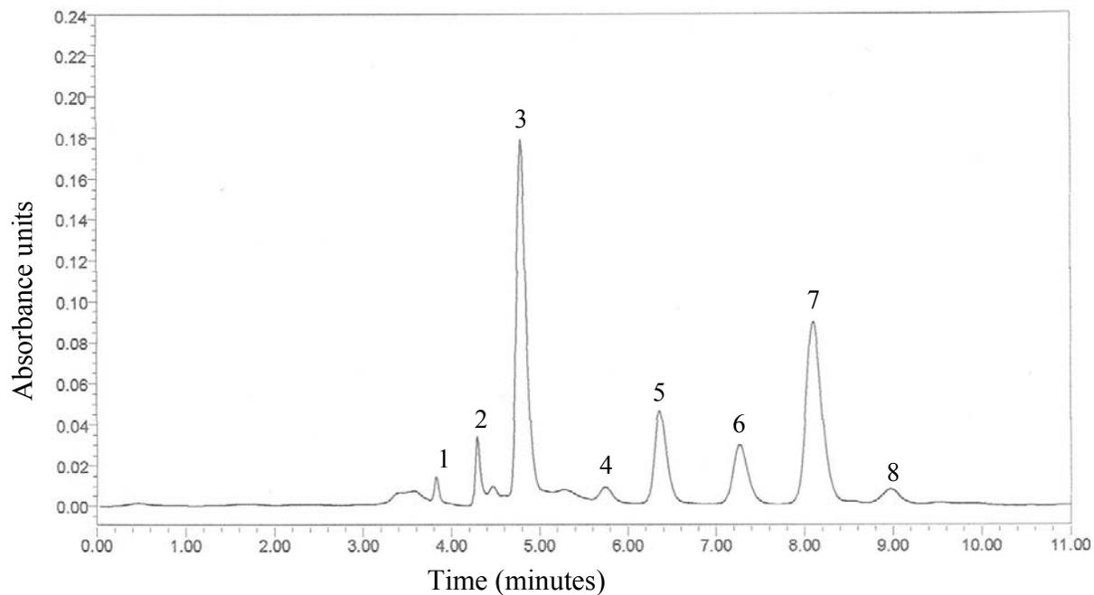
Figure 2.4. A representative chromatogram for a 20 µl sweetpotato extract analyzed with a Gemini C18, 5 µm, 4.6 × 250 mm column using a mobile phase consisting 1% (v/v) formic acid in aqueous solution: acetonitrile: 2-propanol (70:22:8), pH 2.5; flow rate: 0.75 ml/min, temperature: 30 °C, UV detection at 320 nm. Peaks: (1) methanol, (2&4) unknown, (3) chlorogenic acid, (5) caffeic acid, (6) 4,5-dicaffeoylquinic acid, (7) 3,5-dicaffeoylquinic acid, (8) 3,4-dicaffeoylquinic acid.
