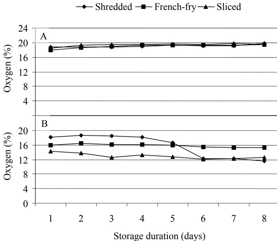
Figure 6.1. Changes in headspace O<sub>2</sub> levels in minimally processed sweetpotatoes stored during storage at 0 °C (A) and 5 °C (B). Each data point represents the mean value of 5 replications.
