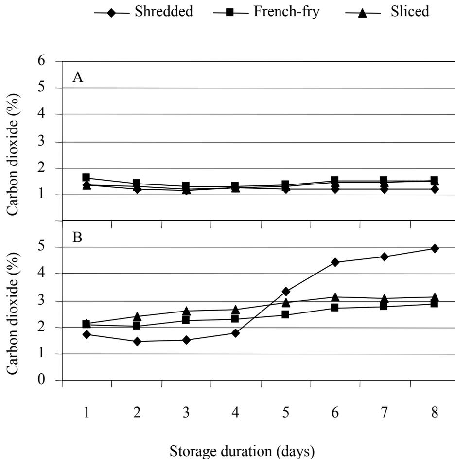
Figure 6.2. Changes in headspace CO<sub>2</sub> levels in minimally processed sweetpotatoes stored during storage at 0 °C (A) and 5 °C (B). Each data point represents the mean value of 5 replications.
