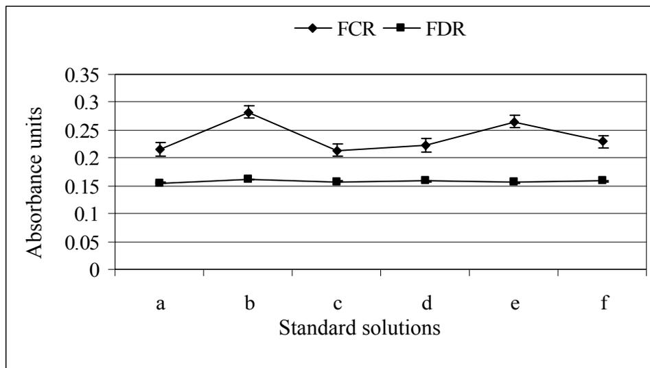
Figure 2.1. Absorbance of standard solutions measured with FDR (Folin-Denis reagent) and FCR (Folin-Ciocalteu reagent). a: 100  $\mu\text{g/ml}$  chlorogenic acid; b: a + 0.05% ascorbic acid; c: a + 4% sucrose; d: a + 2% fructose; e: a + 2% glucose; f: a + 10% maltose. Vertical bars represent standard error of the mean ( $n=5$ ) and, if absent, covered by the symbol.
