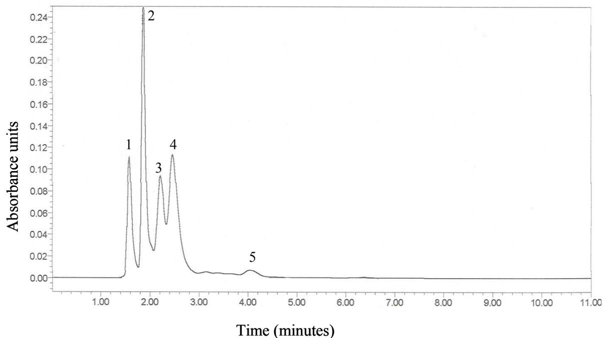
Figure 2.7. A representative HPLC chromatogram for a 20  $\mu$ l sweetpotato extract analyzed with a Novapak C18, 4  $\mu$ m, 3.9  $\times$  150 mm column using a mobile phase consisting 1% (v/v) formic acid in aqueous solution: acetonitrile: 2-propanol (70:22:8), pH 2.5; flow rate: 0.75 ml/min, temperature: 30  $^{\circ}$ C, UV detection at 320 nm. Peaks: (1) methanol, (2) chlorogenic acid, (3) caffeic acid, (4) 3,5-dicaffeoylquinic acid, (5) unknown.
