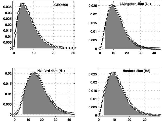
FIG. 6. Measured pdf for  $2\mathcal{F}$  for all four interferometer data with injected signals as described in Table III. The circles represent the measured PDF values from the Monte Carlo simulations. The lines represent  $\chi^2$  distributions with four degrees of freedom and best-fit noncentrality parameters given in Table III. The filled area represents the integral of the pdfs between  $2\mathcal{F}^*$  and  $+\infty$ .
