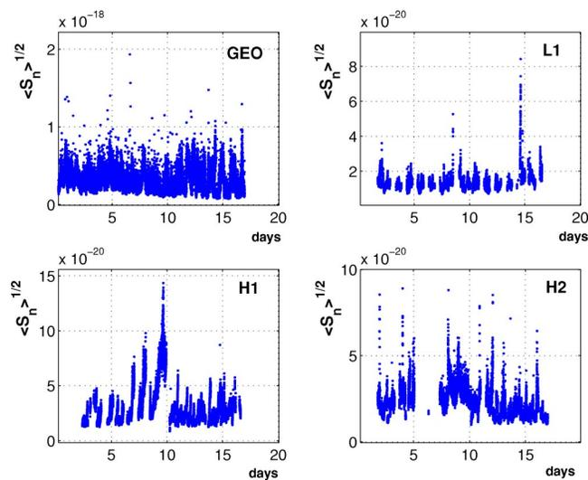
FIG. 4. The square root of the average value of  $S_n$  for all four interferometers over a band of 1 Hz starting at 1283.5 Hz versus time in days starting at the beginning of S1 (23 August 2002, 15:00 UTC).
