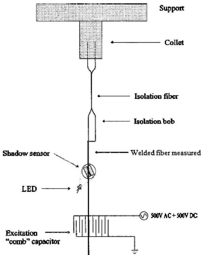
FIG. 2. Schematic of the ringdown experiment. The bob to which the fiber is welded is attached to another silica bob above it by a silica fiber.
