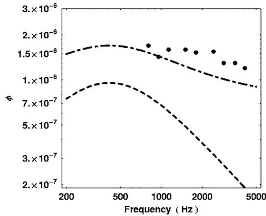
FIG. 4. Measured dissipation against resonance frequency of the welded fiber. The points are the measured loss angles, the dashed line is thermoelastic damping for a  $65 \mu\text{m}$  silica fiber, while the solid line shows the expected loss from thermoelastic damping and structural surface loss for the same diameter. The thermoelastic peak has been reduced by 0.65, in line with results from other measurements.
