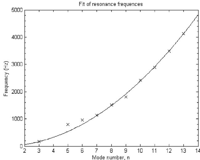
FIG. 3. Fit of measured modal frequency data to the model of resonances of a circular cross-section, fused silica fiber. The fiber was measured to have a length of  $80 \pm 2$  mm and diameter of  $65 \pm 5$   $\mu\text{m}$ . The continuous line is meant to simply guide the eye and has no significance between integers.
