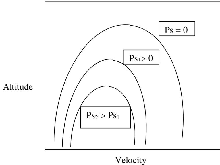
Figure 5.2. Specific Energy Rate for Typical Fighter Aircraft
